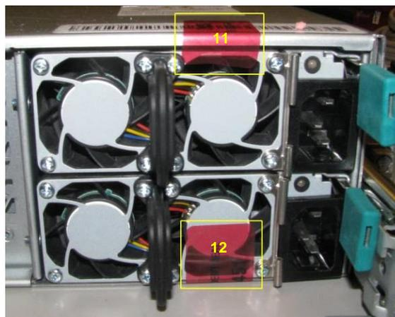
Figure 19 – Tamper-Evident Seal Application Positions (S5032 / S6032 – Rear)
