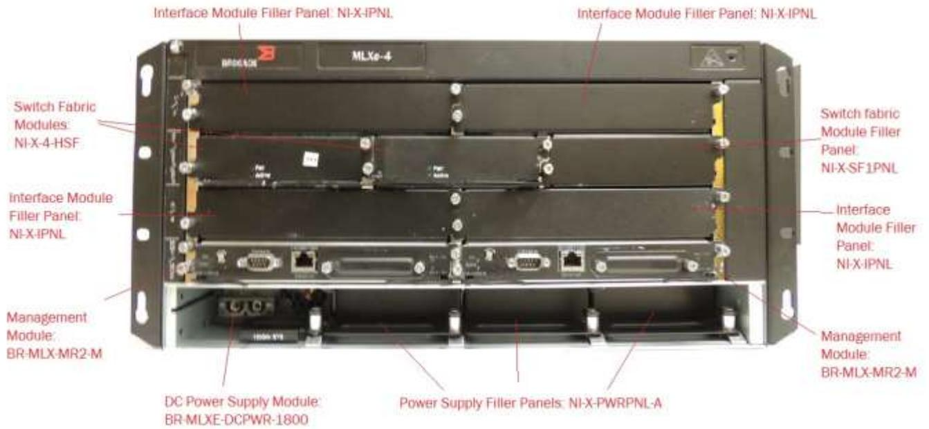
Figure 8 MLXe-4 Cryptographic Module with Chassis: BR-MLXE-4-MR2-M-DC backside
