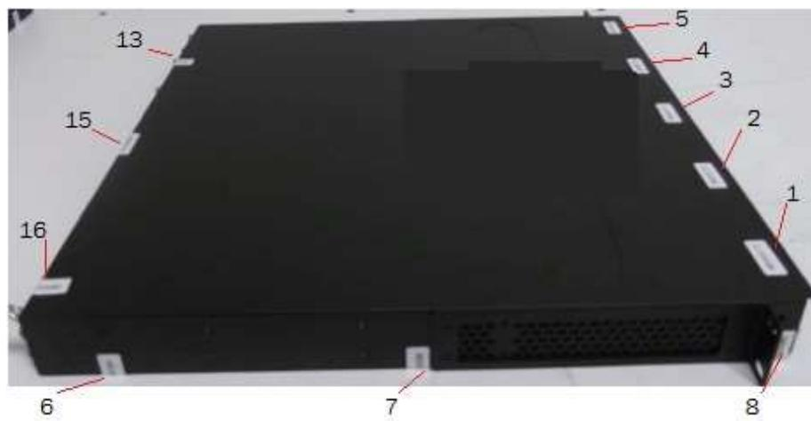
**Figure 95 Rear view of a Brocade CER 2024C-4X-RT device with security seals**
