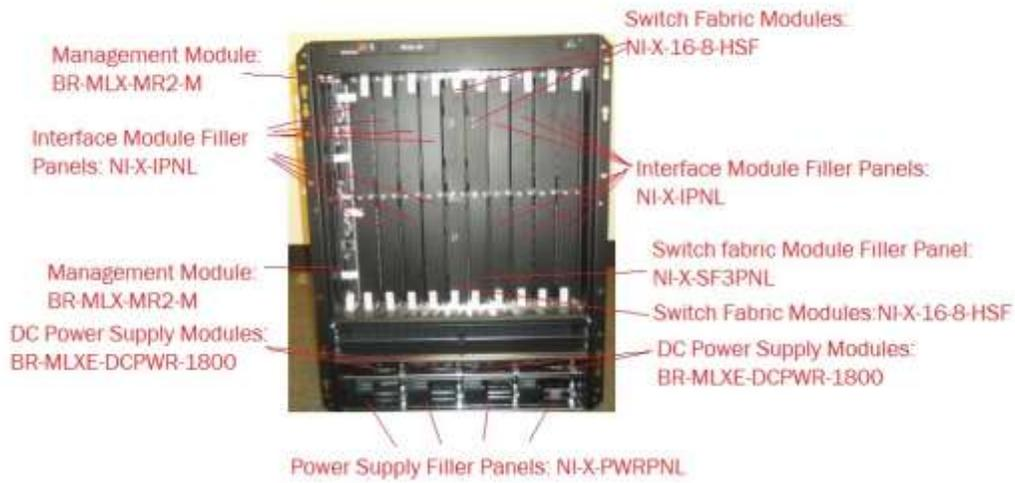
Figure 24 MLXe-16 Cryptographic Module with Chassis: BR-MLXE-16-MR2-M-DC backside
