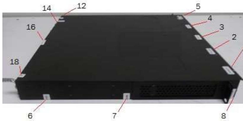
**Figure 110 Rear view of a Brocade CES 2024F-4X device with security seals**
