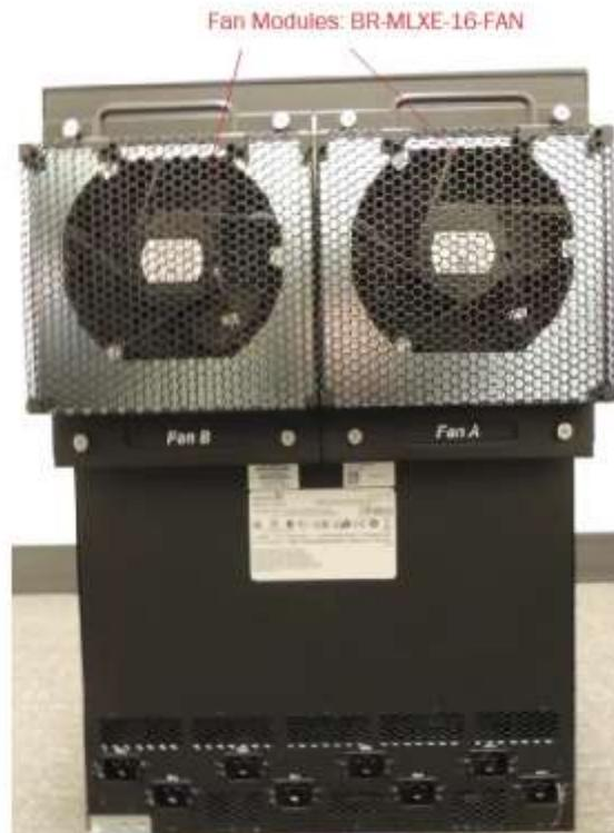
Figure 19 MLXe-16 Cryptographic Module with Chassis: BR-MLXE-16-MR-M-DC (DC Power Supply)
