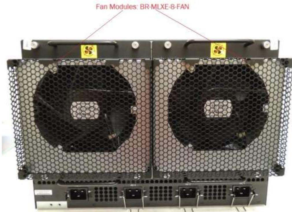
Figure 17 MLXe-16 Cryptographic Module with Chassis: BR-MLXE-16-MR-M-AC (AC Power supply)
