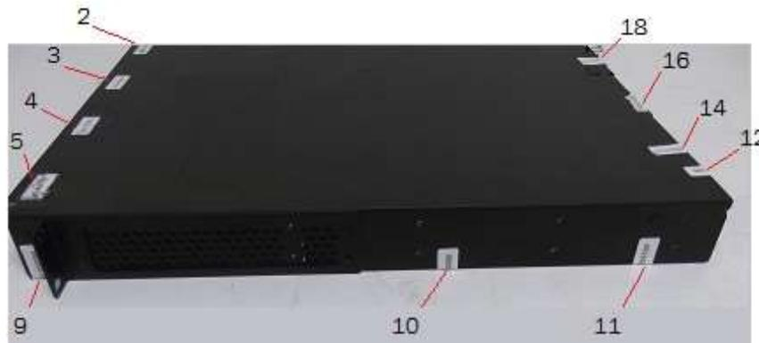
**Figure 104 Left side view of a Brocade CES 2024C-4X device with security seals**
