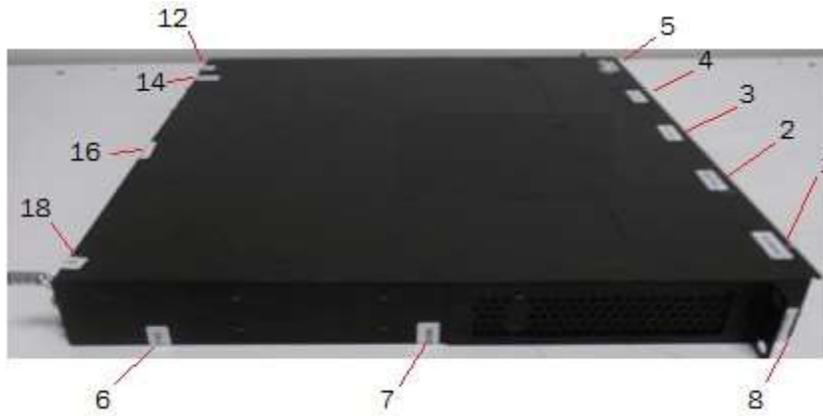
**Figure 105 Rear view of a Brocade CES 2024C-4X device with security seals**
