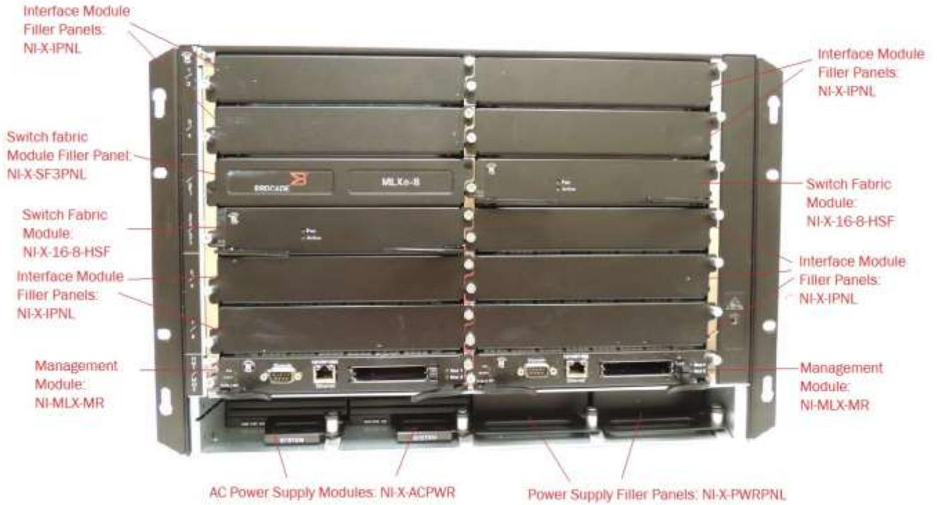
Figure 10 MLXe-8 cryptographic module with Chassis: BR-MLXE-8-MR-M-AC backside
