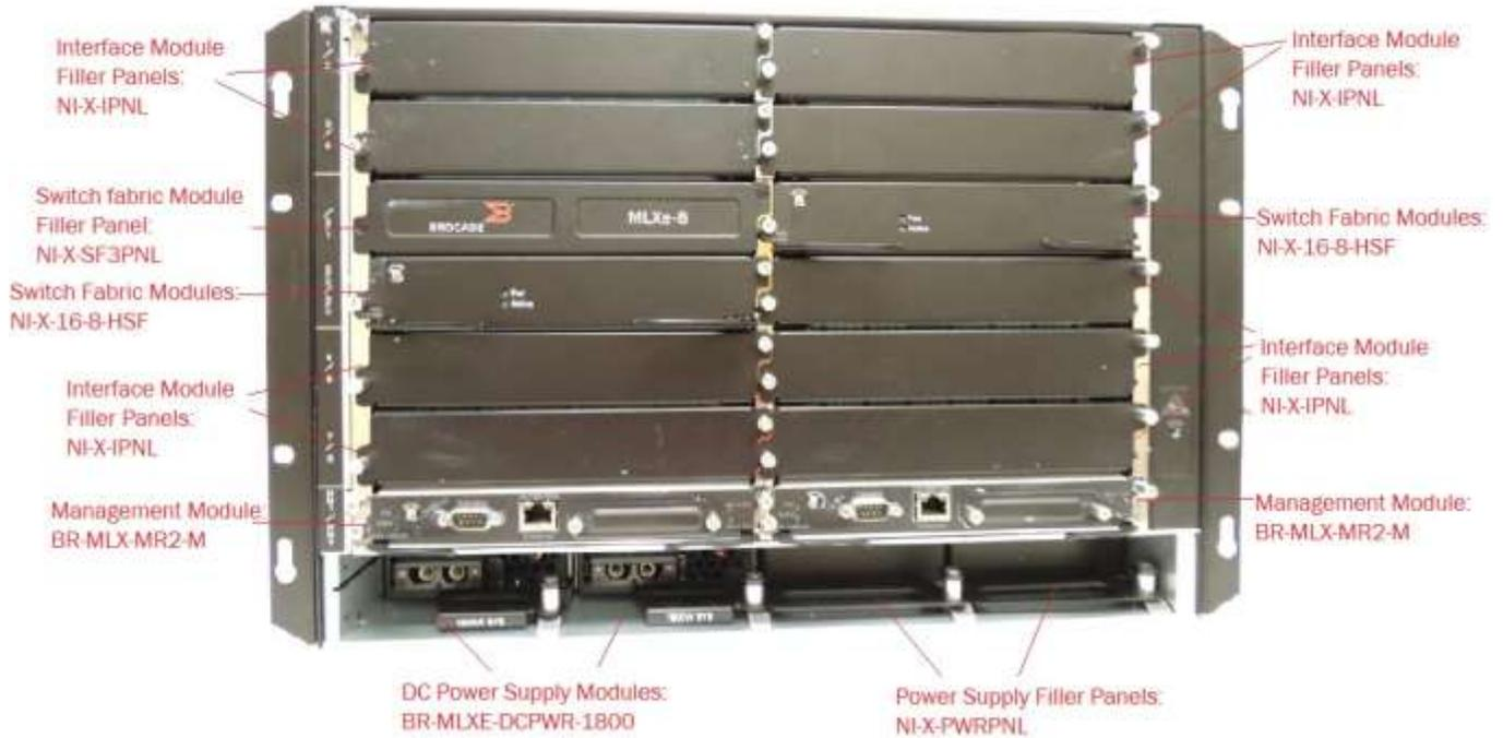
Figure 16 MLXe-8 Cryptographic Module with Chassis: BR-MLXE-8-MR2-M-DC backside
