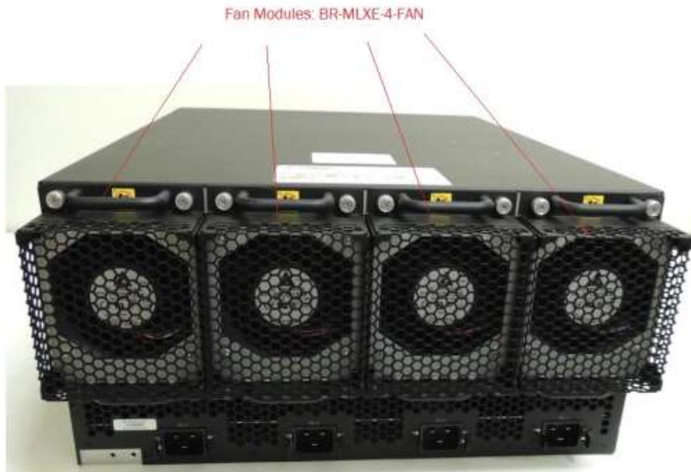
Figure 5 MLXe-4 Cryptographic Module with Chassis: BR-MLXE-4-MR2-M-AC (AC Power Supply)
