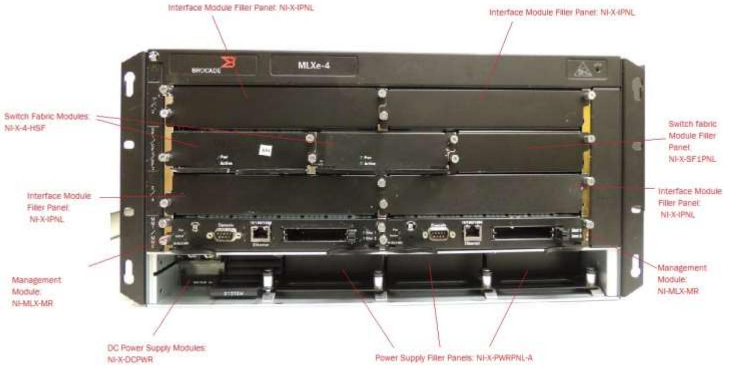
Figure 4 MLXe-4 Cryptographic Module with Chassis: BR-MLXE-4-MR-M-DC backside
