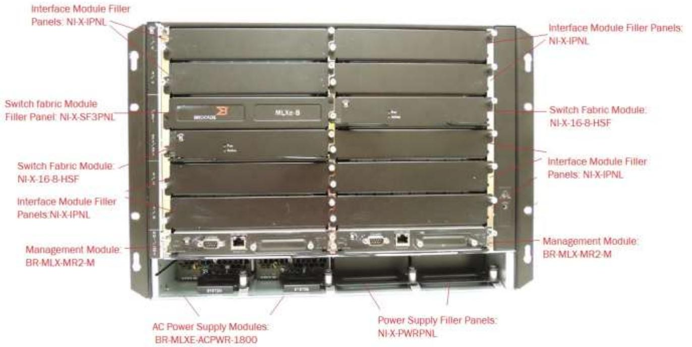
Figure 14 MLXe-8 Cryptographic Module with Chassis: BR-MLXE-8-MR2-M-AC backside
