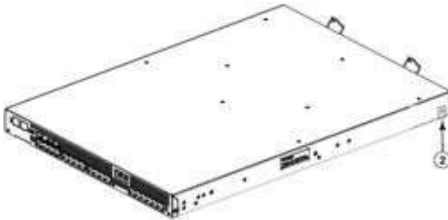
Figure 26 Brocade 7800 top right port side seal locations
