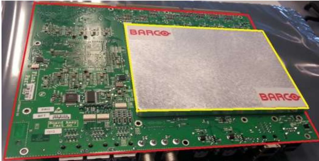
Picture 1 – Barco ICMP main board bottom view
