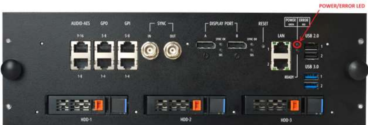
Picture 7 – Barco ICMP full assembly front panel with highlighted Power/Error LED
