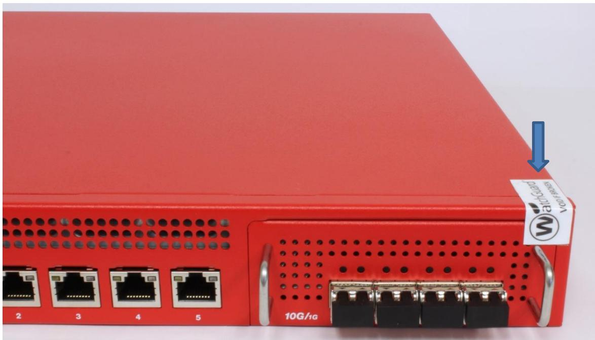
Figure 13: WatchGuard XTM 1525, 1525-RP Front Panel Tamper Evident Label Placement
