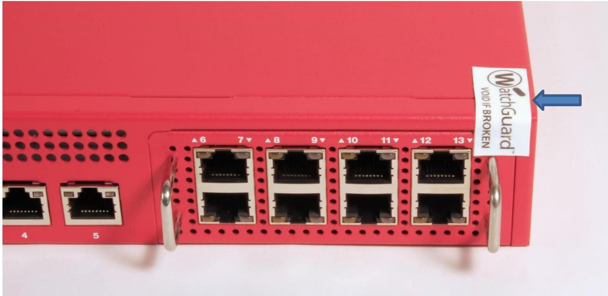
Figure 9: WatchGuard XTM 850, 860, 870 Front Panel Tamper Evident Label Placement
