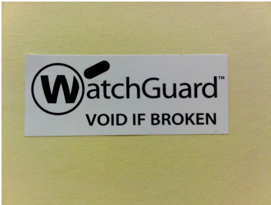
**Figure 8: WatchGuard XTM Tamper Evident Label**
