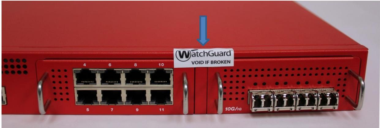
Figure 16: WatchGuard XTM 2500 Series Front Panel Tamper Evident Label Placement
