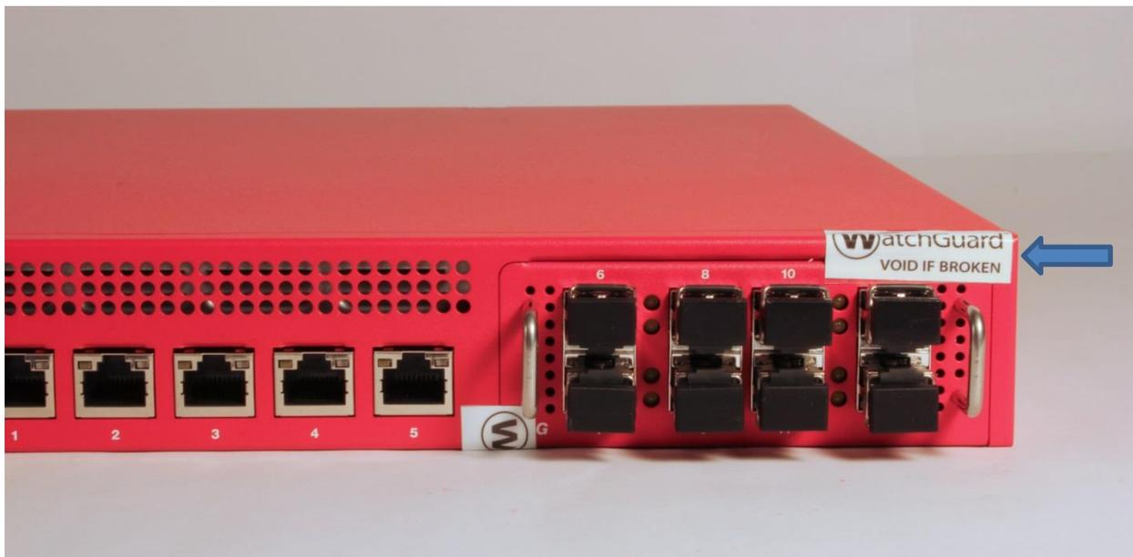
Figure 10: WatchGuard XTM 870-F Front Panel Tamper Evident Label Placement
