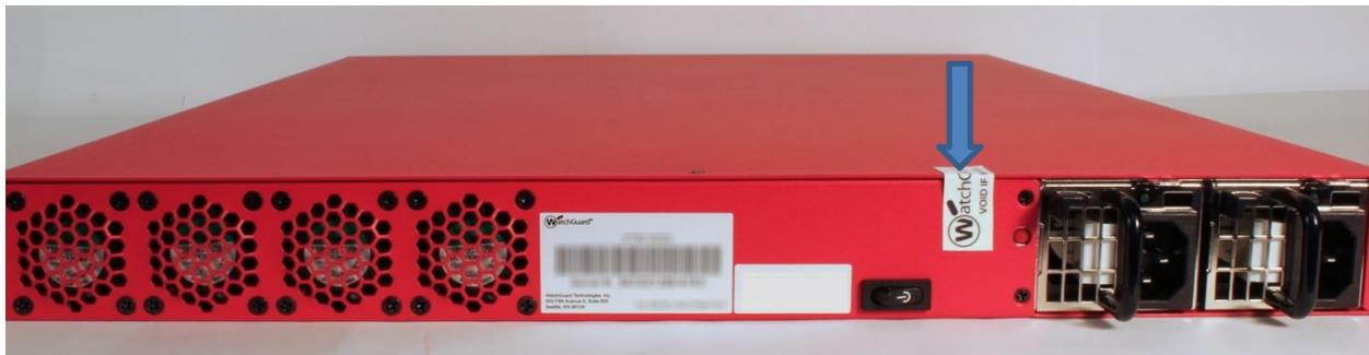
Figure 17: WatchGuard XTM 2500 Series Rear Panel Tamper Evident Label Placement
