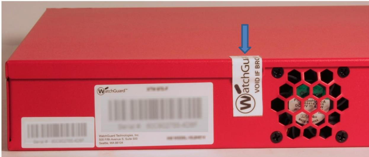
**Figure 11: WatchGuard XTM 800 Series Rear Panel Tamper Evident Label Placement**
