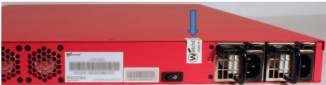
**Figure 15: WatchGuard XTM 1520-RP, 1525-RP Series Rear Panel Tamper Evident Label Placement**
