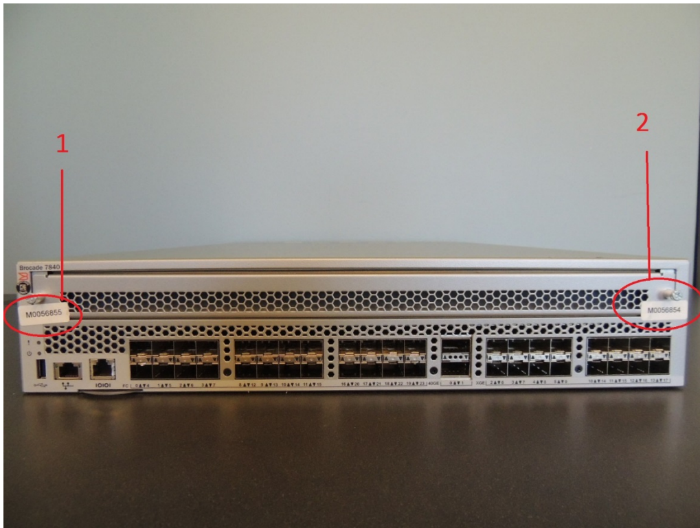
Figure 29: Brocade 7840 front side seal locations (QTY 2)
