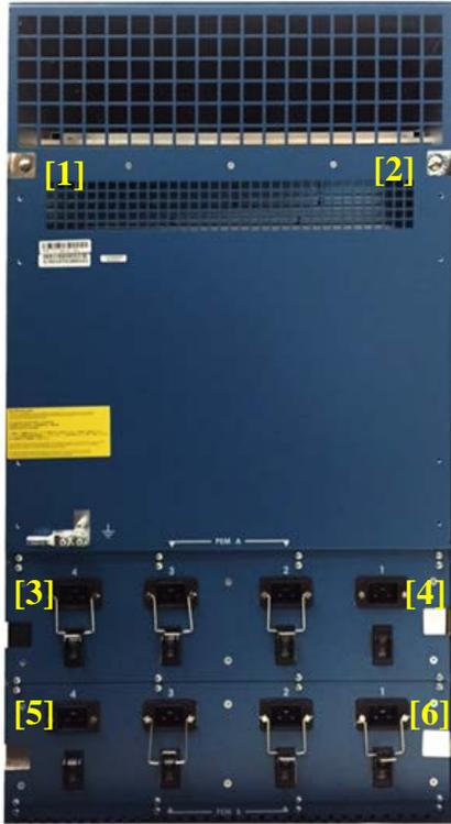
**Figure 13 - PA-7080 Tamper Seal Placement for Rear (6)**
