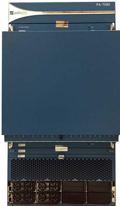
Figure 6 - PA-7080 Front with Opacity Shield
