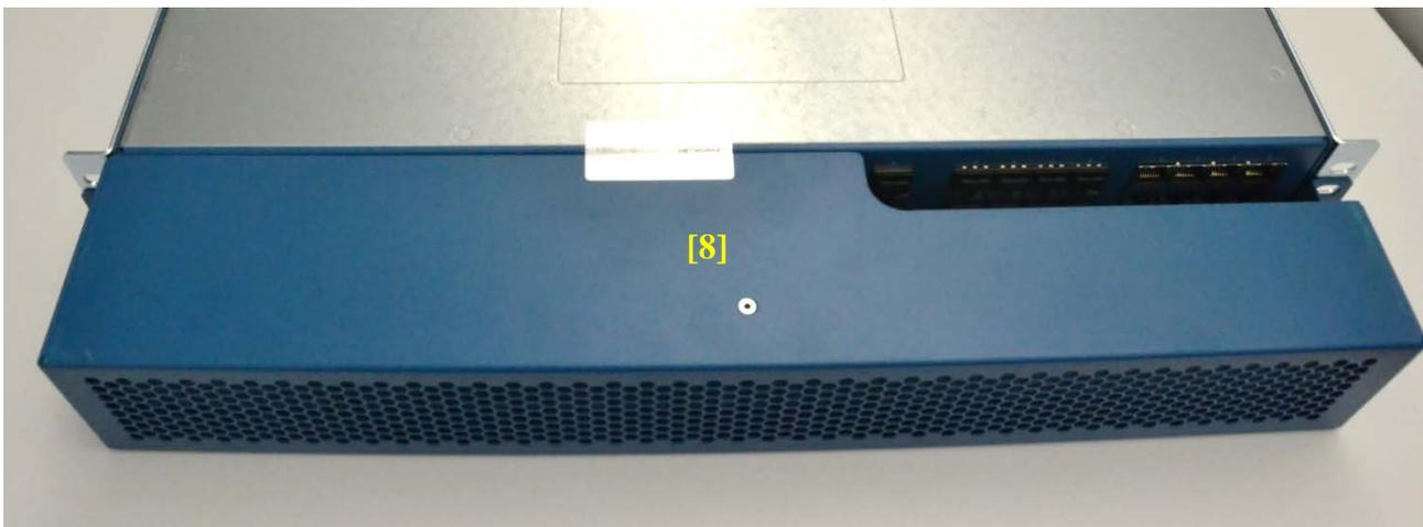
Figure 12 – PA-3060 Front/Bottom Tamper Seal Placement
