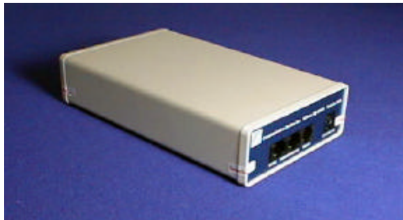
Figure 6 UniGuard-V90 with Tamper Tape seals on rear and side of unit
