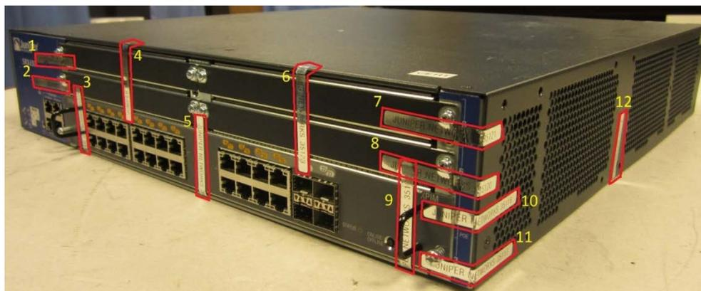
**Figure 22: SRX650 Tamper-Evident Seal Placement on Front and Right Side- Twelve Seals**
