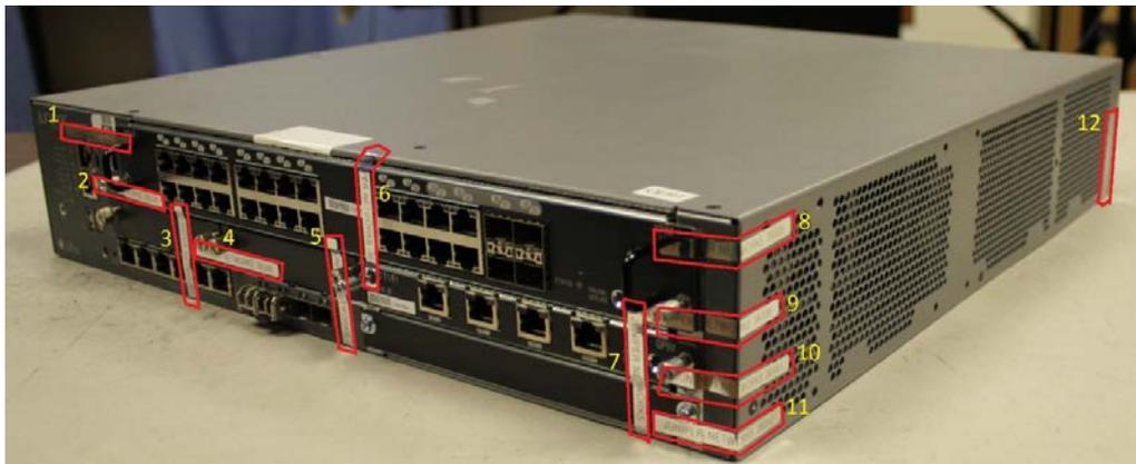
**Figure 20: SRX550 Tamper-Evident Seal Placement on Front and Right Side-Twelve Seals**
