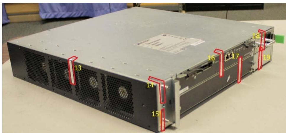
**Figure 23: SRX650 Tamper-Evident Seal Placement on Rear and Left Side- Seven Seals**
