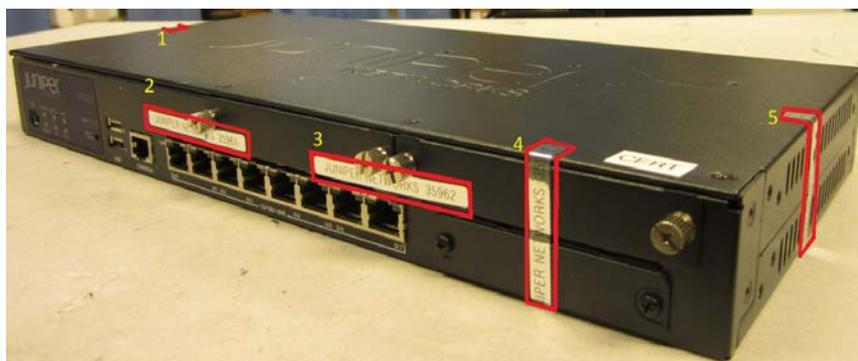
**Figure 18: SRX220 Tamper-Evident Seal Placement- Five Seals**
