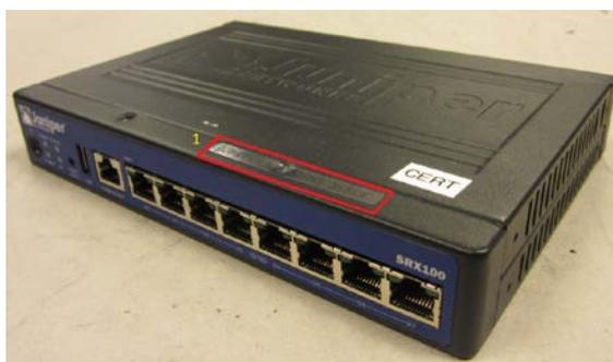
**Figure 15: SRX100 Tamper-Evident Seal Placement- One Seal**
