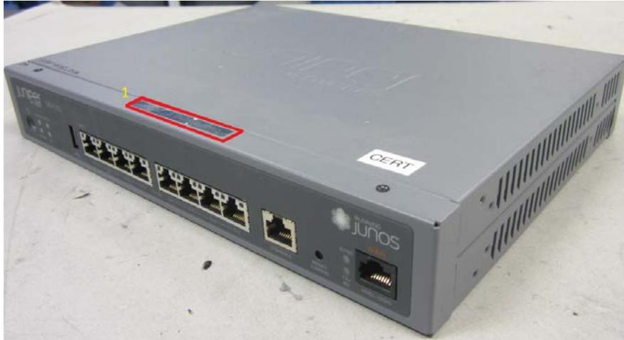
Figure 16: SRX110 Tamper-Evident Seal Placement- One Seal
