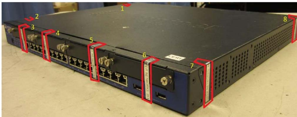
**Figure 19: SRX240 Tamper-Evident Seal Placement-Eight Seals**
