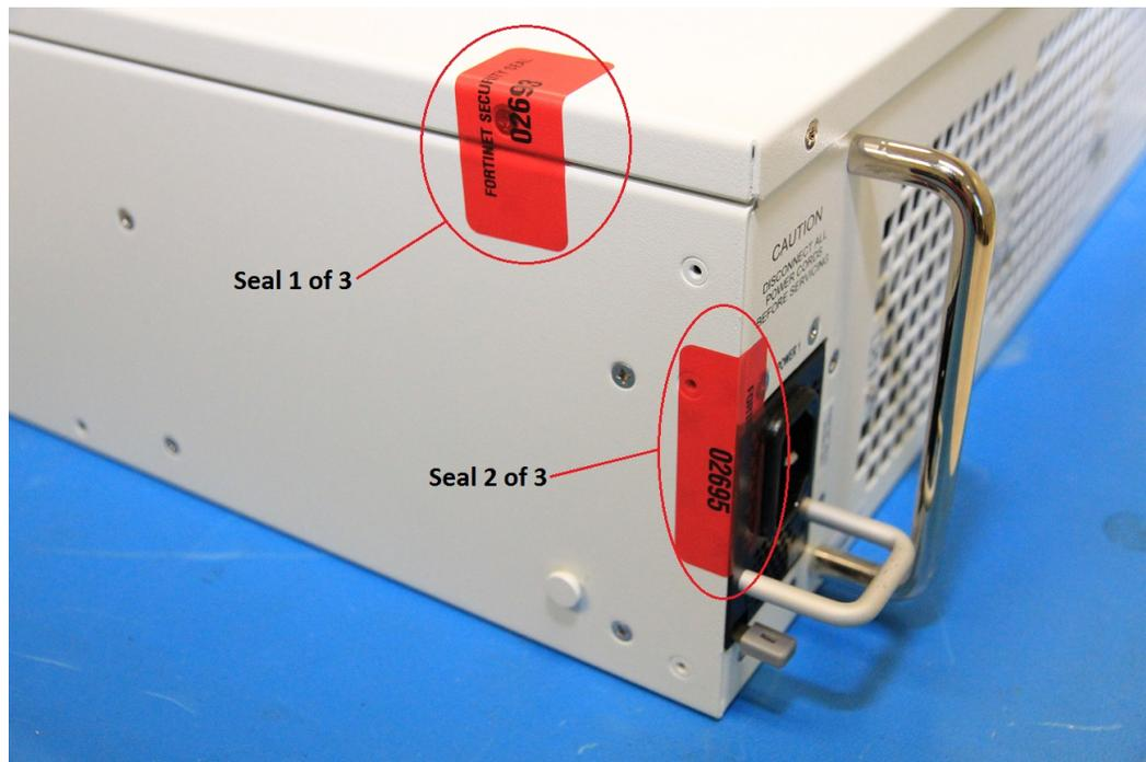
Figure 5: FortiGate-3700D Power Supply Seal, rear, left side
