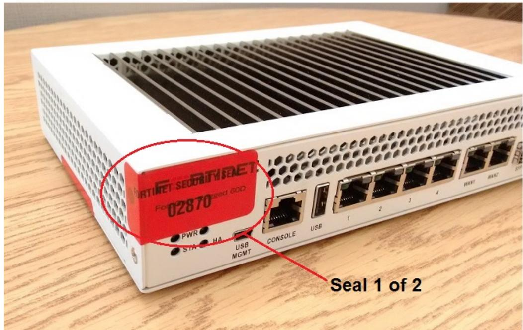
Figure 12: FortiGate-92D external enclosure seal, bottom, left side
