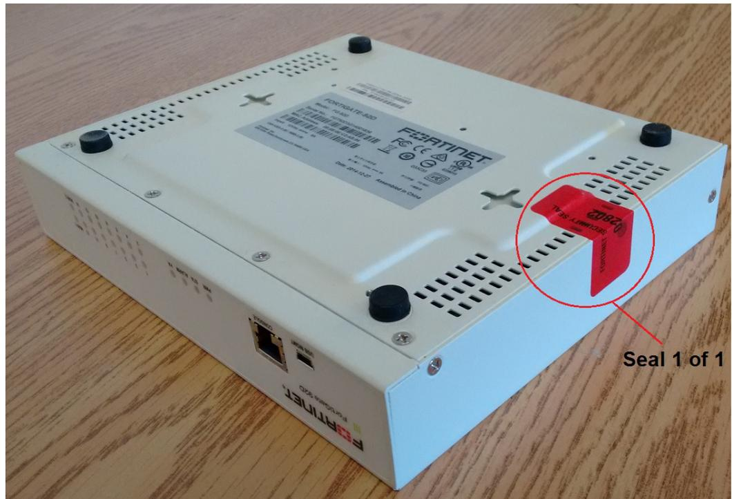
Figure 11: FortiGateRugged-60D front panel seal
