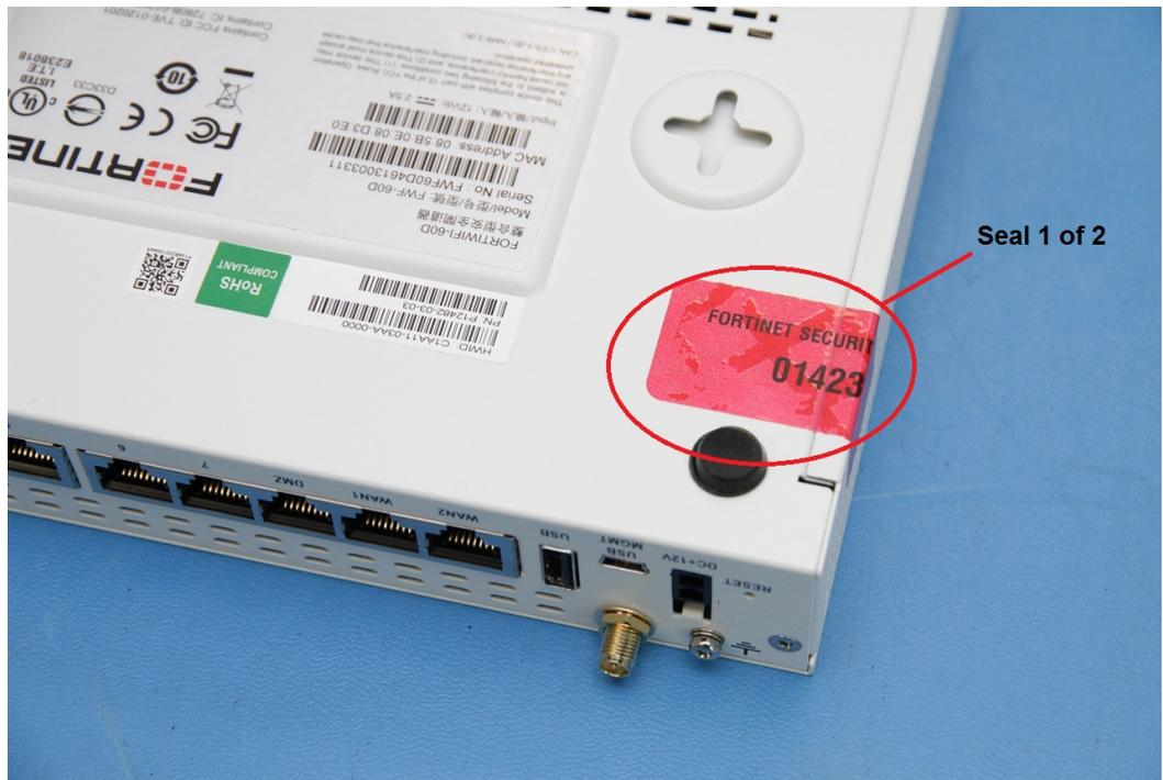
Figure 9: FortiWiFi-60D external enclosure seal, top, rear
