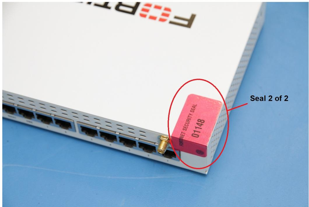
Figure 10: FortiGate-92D external enclosure seal, bottom, left side
