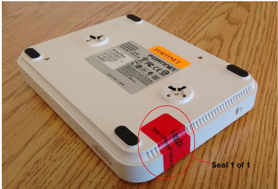
Figure 8: FortiWiFi-60D external enclosure seal, bottom, right side
