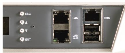
Figure 16 – RJ45 Ethernet, Console and USB close-up
