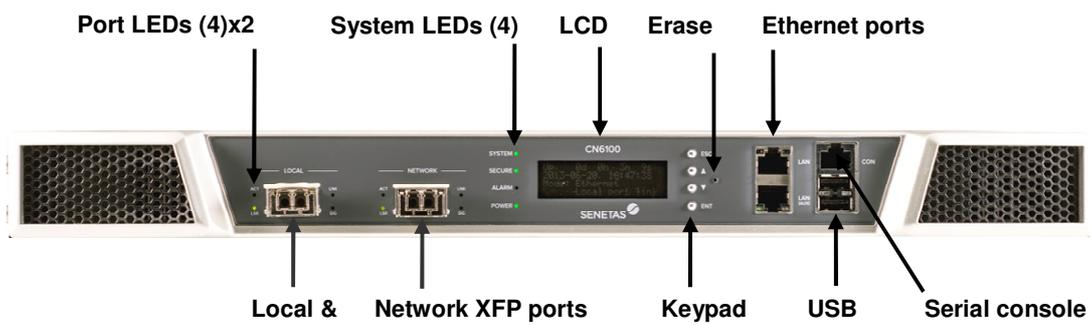
Figure 12 - Front View of the CN6100 [O] Encryptor
