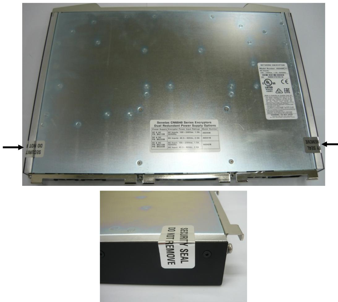
Figure 17 – Factory installed tamper seals
