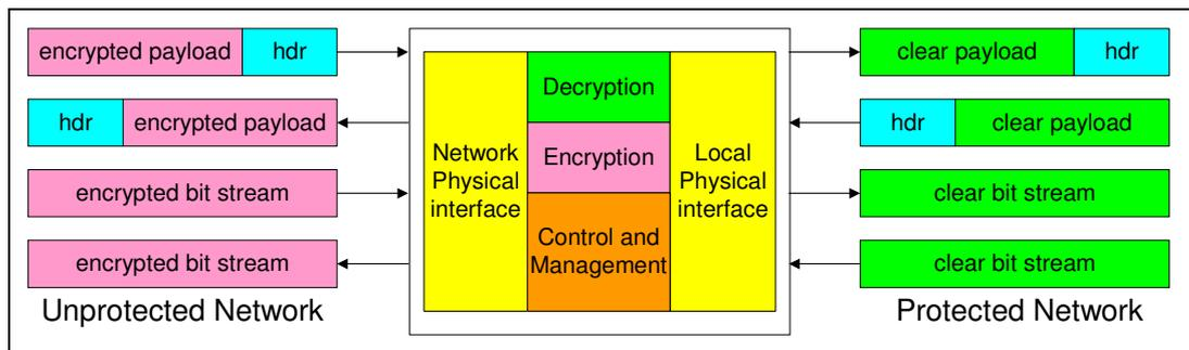
**Figure 3 - Data Flow through the Encryptor**
