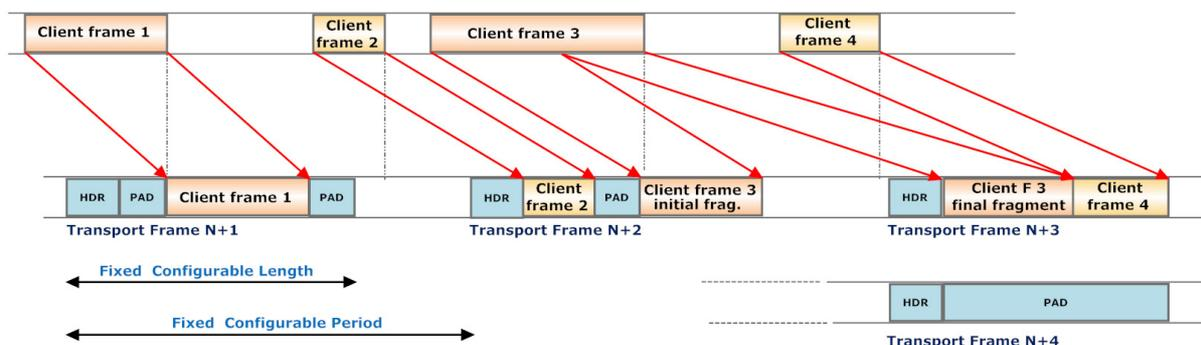
Figure 7 – TRANSEC constant rate transport frame assembly
