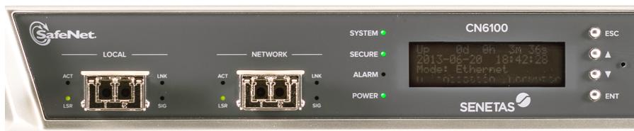
Figure 14 – A6100B [Y] 10G Ethernet port close-up - XFPs installed
