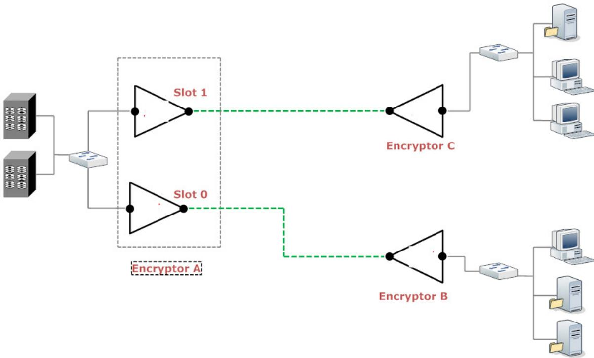
Figure 7 – Fibre Channel Configuration
