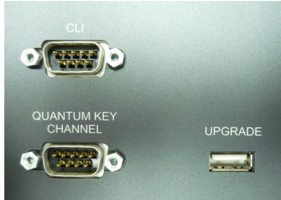
**Figure 12 – Serial ports and USB close-up**
