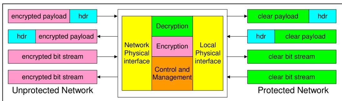
Figure 3 - Data Flow through the Encryptor slot
