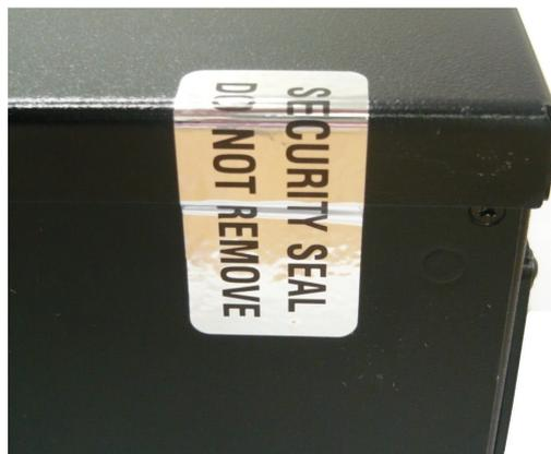
**Figure 14 – Factory installed tamper seal close-up**
