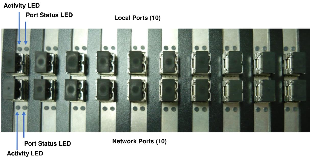
Figure 10 – CN8000 Slots close-up – SFP+s installed
