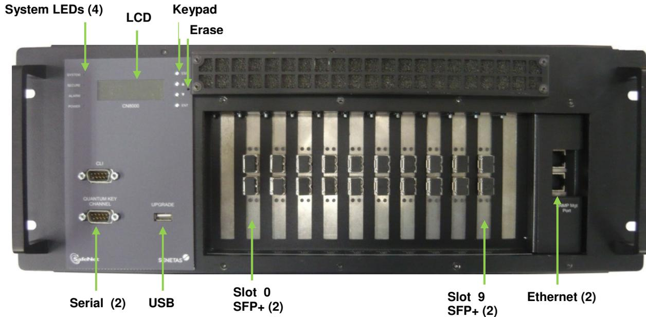
Figure 8 - Front View of the CN8000 Encryptor
