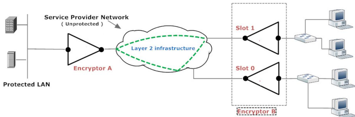
**Figure 5 - Meshed Configuration**
