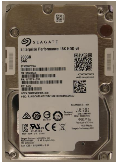
Enterprise Performance® HDD v6, 2.5", 15K-RPM, SAS Interface, 900GB, 600GB
