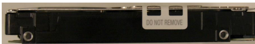
Figure 5: Left-side view of tamper-evidence label on left side of Enterprise Performance HDD v6, 2.5-Inch, 15K-RPM, SAS Interface module
