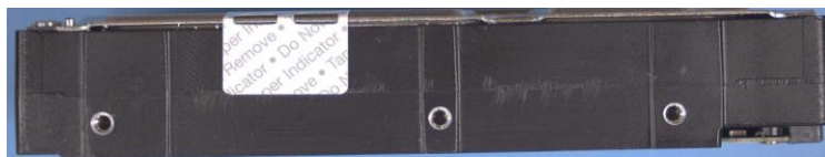
Figure 3: Right-side view of tamper-evidence label on right side of Enterprise Performance HDD v1, 3.5-inch, 10K-RPM, SAS Interface module
