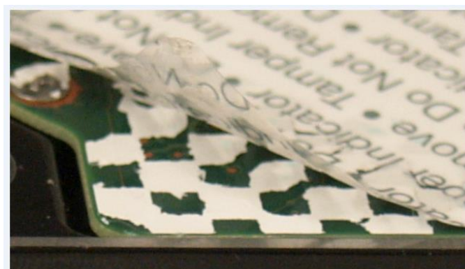
Figure 11: Enterprise Performance HDD v1, 3.5-inch, 10K-RPM, SAS Interface, Enterprise Performance HDD v6, 2.5-Inch, 15K-RPM, SAS Interface, Enterprise Capacity HDD v6, 3.5-inch, 7K-RPM, SAS Interface module PCBA Tamper Evidence. Label lifted off.
