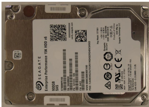
Figure 4: Top view of tamper-evidence label on sides of Enterprise Performance HDD v6, 2.5-Inch, 15K-RPM, SAS Interface module
