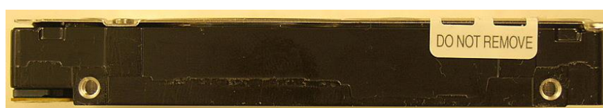
Figure 8: Left-side view of tamper-evidence label on left side of Enterprise Performance HDD v9, 2.5-Inch, 10K-RPM, SAS Interface module
