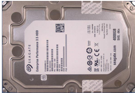
Figure 1: Top view of tamper-evidence label on sides of Enterprise Performance HDD v1, 3.5-inch, 10K-RPM, SAS Interface module
