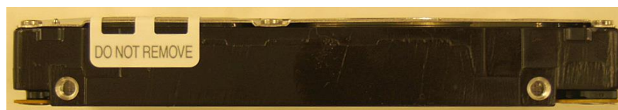
Figure 9: Right-side view of tamper-evidence label on right side of Enterprise Performance HDD v9, 2.5-Inch, 10K-RPM, SAS Interface module
