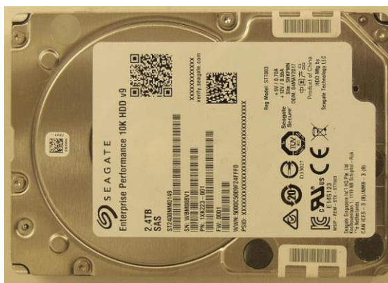
Figure 7: Top view of tamper-evidence label on sides of Enterprise Performance HDD v9, 2.5-Inch, 10K-RPM, SAS Interface module
