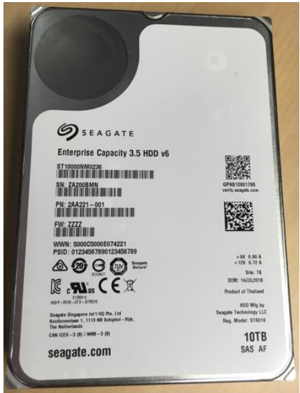
Enterprise Capacity® HDD v6, 3.5", 7K-RPM, SAS Interface, 10,000GB
