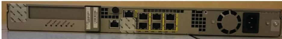
**Figure 45 ASA 5515-X Rear TEL Placement**
