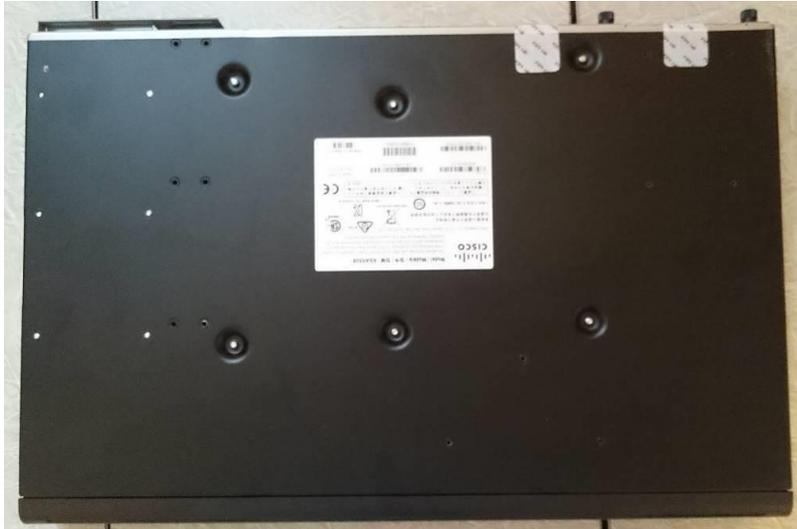
**Figure 36 ASA 5508-X Bottom TEL Placement**
