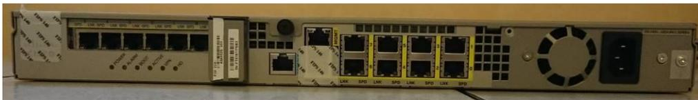
**Figure 57 ASA 5525-X Rear TEL Placement**
