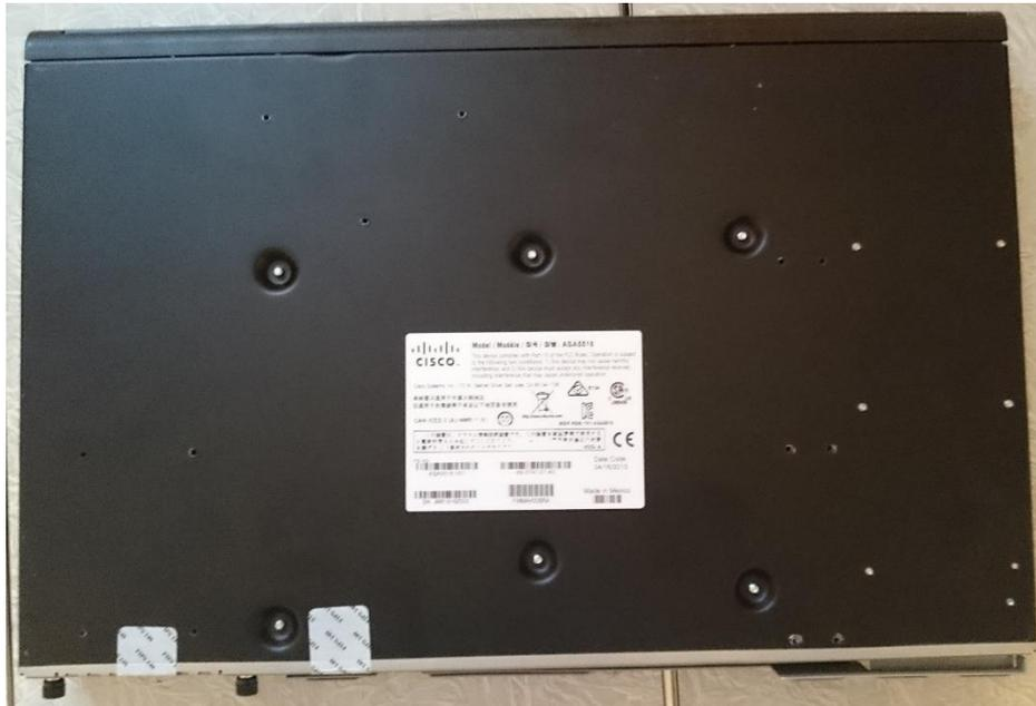
**Figure 54 ASA 5516-X Bottom TEL Placement**
