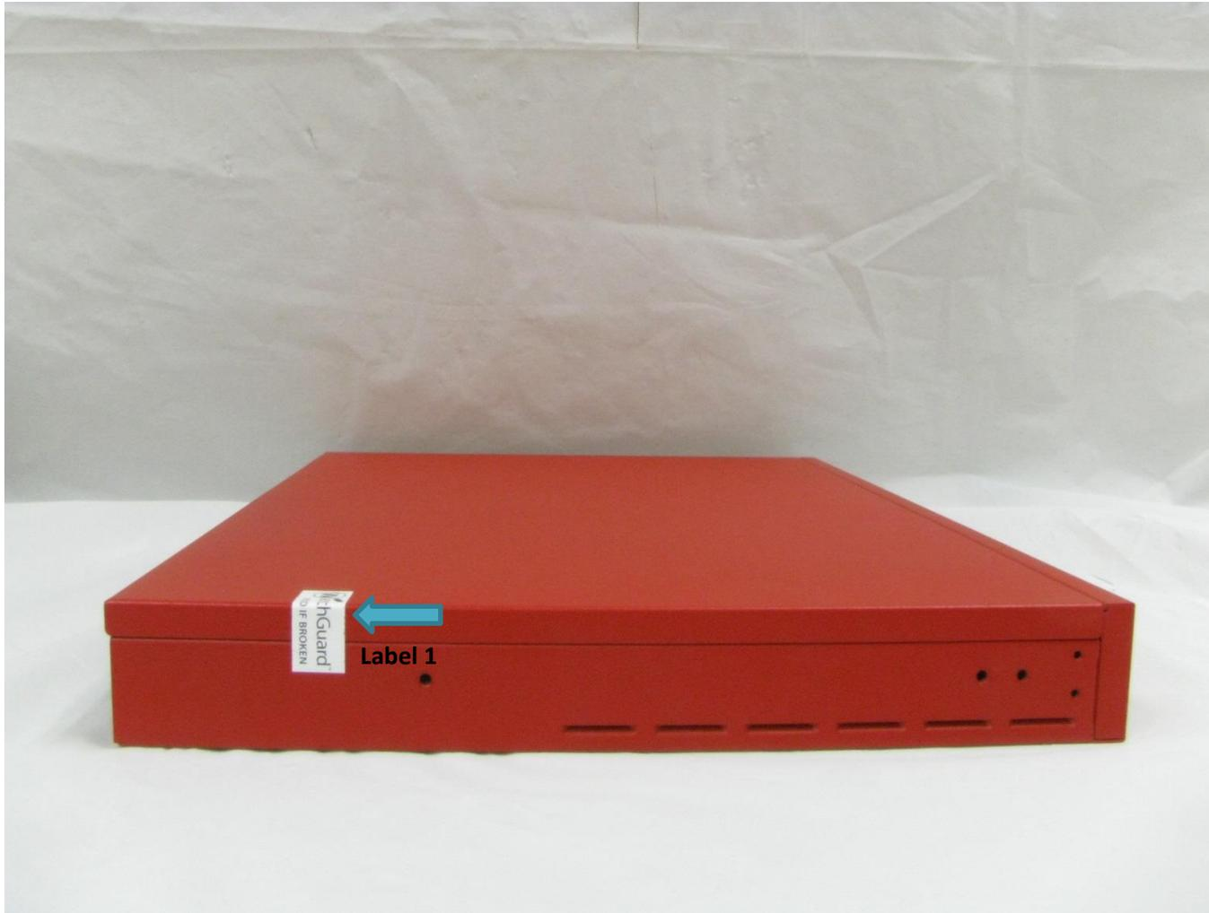
**Figure 14: M300 Tamper Evident Label 1 Placement**
