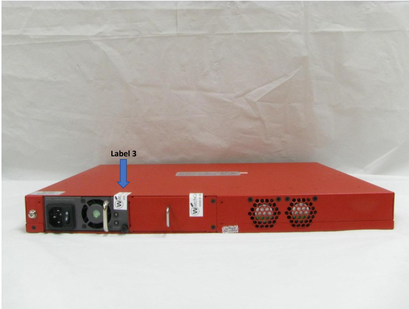
**Figure 19: M440 Tamper Evident Label 3 Placement**
