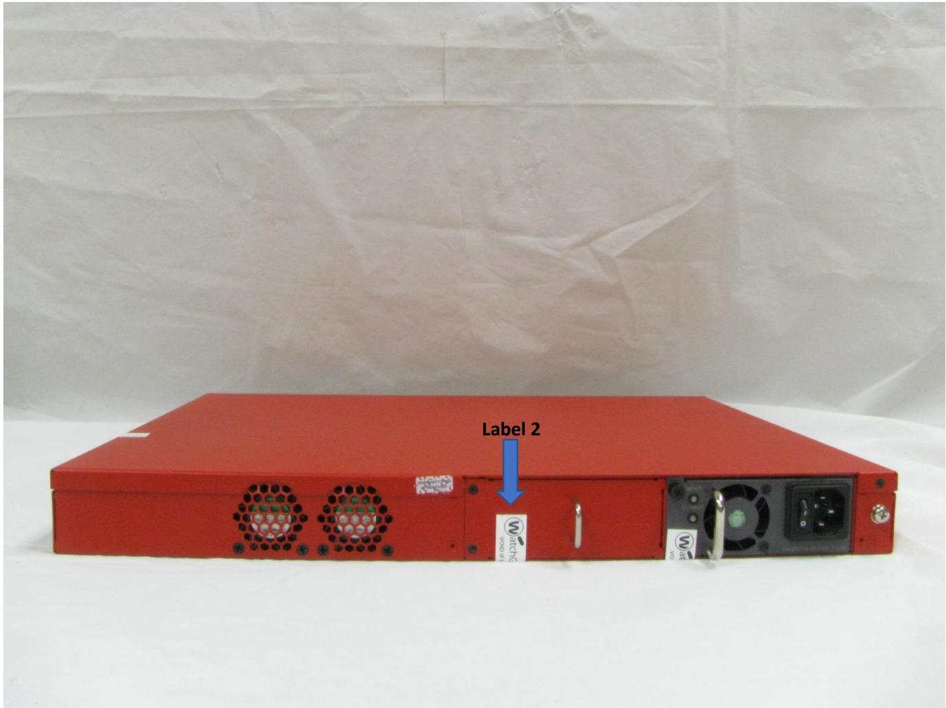
**Figure 18: M440 Tamper Evident Label 2 Placement**
