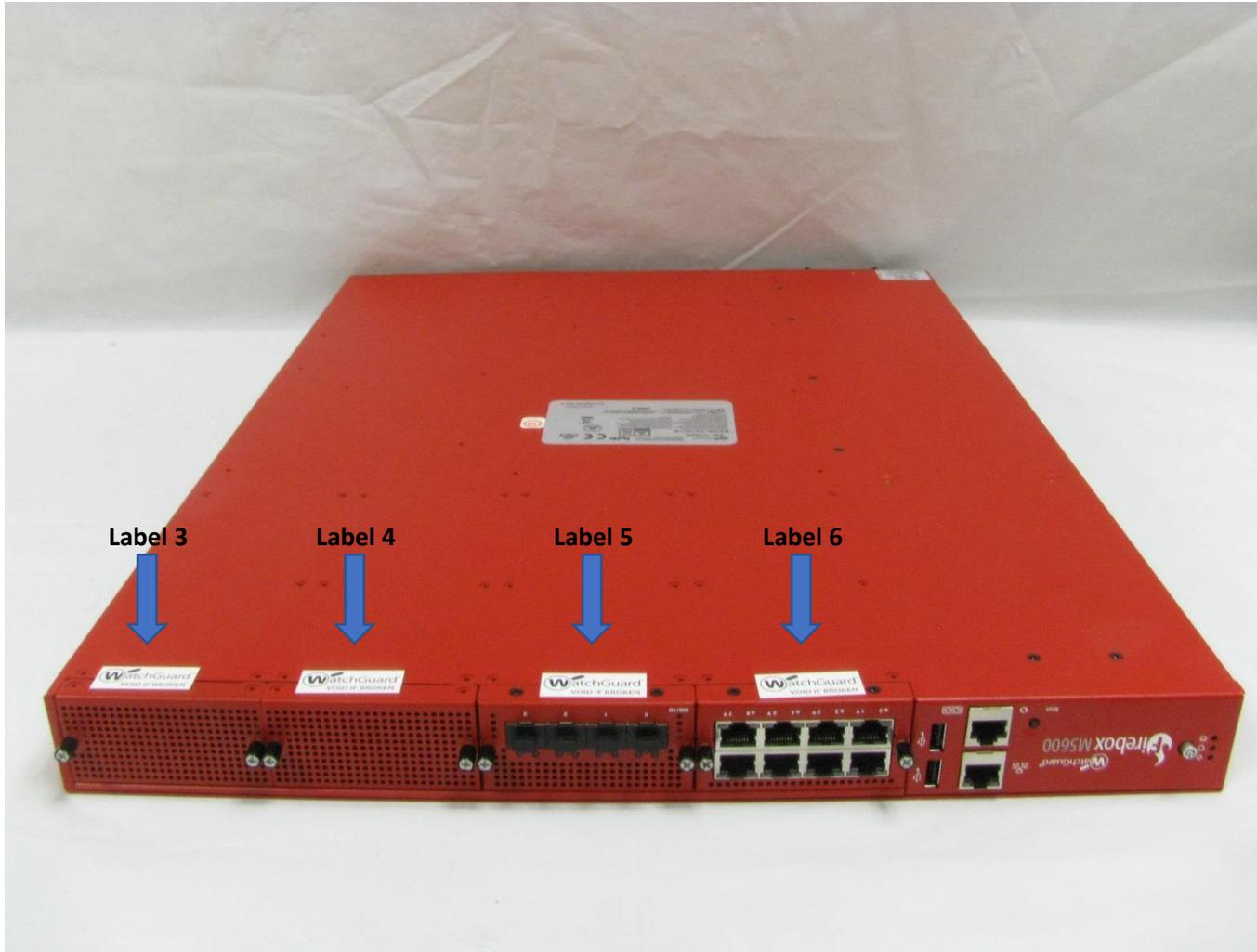
Figure 25: M5600 Tamper Evident Label 3/Label 4/Label 5/Label 6 Placement
