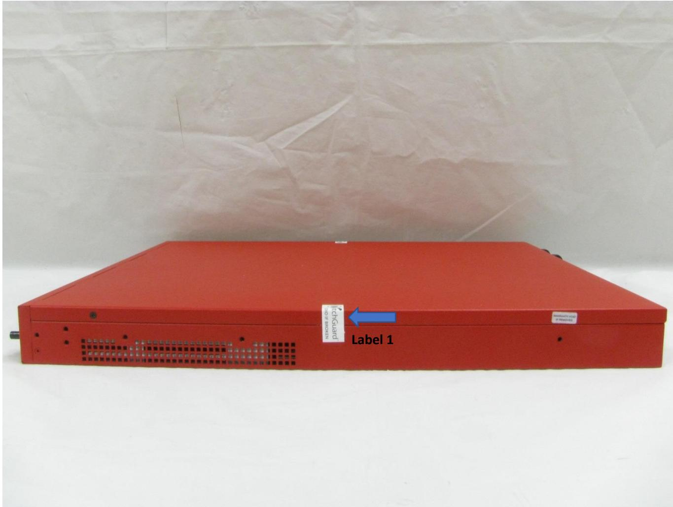
Figure 20: M4600 Tamper Evident Label 1 Placement
