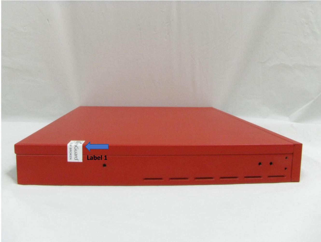
**Figure 13: M200 Tamper Evident Label 1 Placement**
