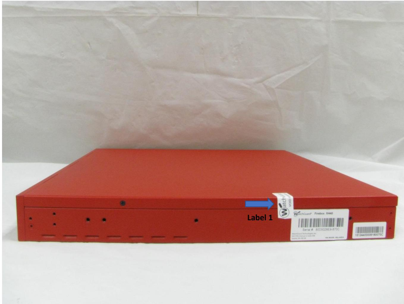
**Figure 17: M440 Tamper Evident Label 1 Placement**
