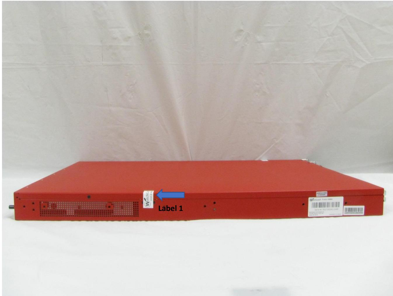
**Figure 23: M5600 Tamper Evident Label 1 Placement**
