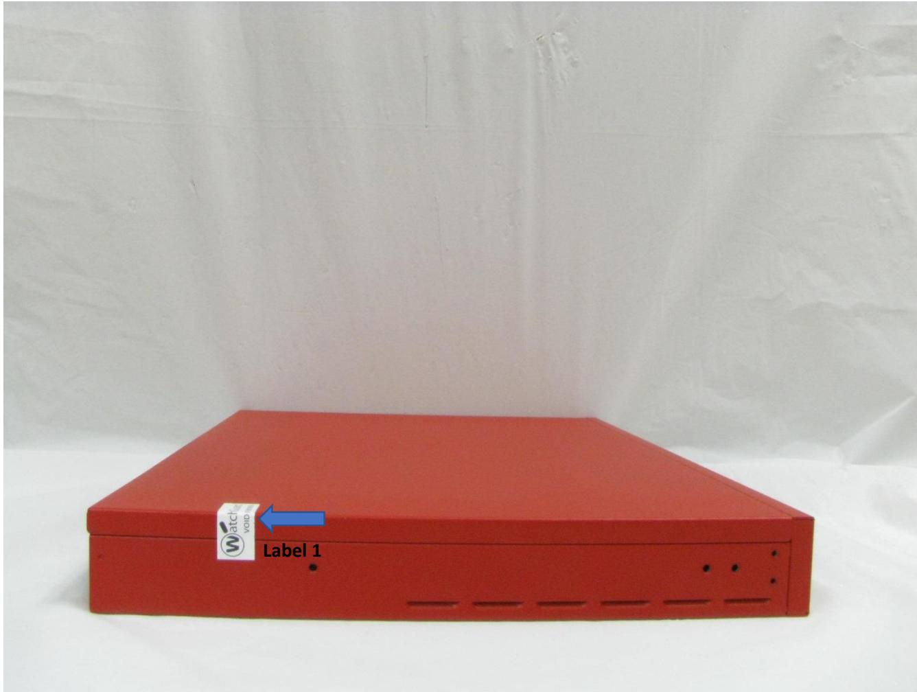
**Figure 16: M500 Tamper Evident Label 1 Placement**
