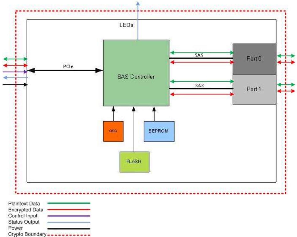
Figure 3 – Block Diagram
