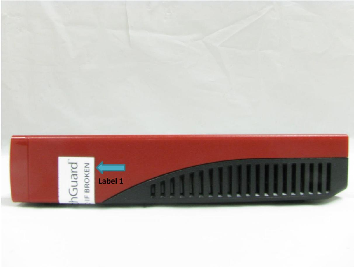
Figure 15: T10 Tamper Evident Label 1 Placement
