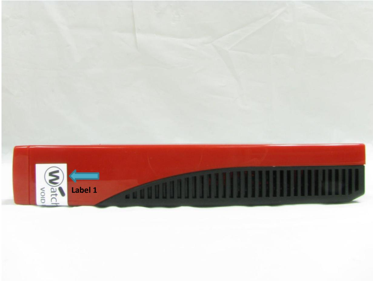
Figure 20: T50-W Tamper Evident Label 1 Placement
