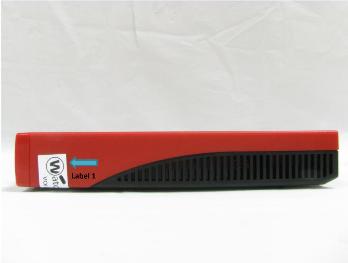
Figure 19: T50 Tamper Evident Label 1 Placement
