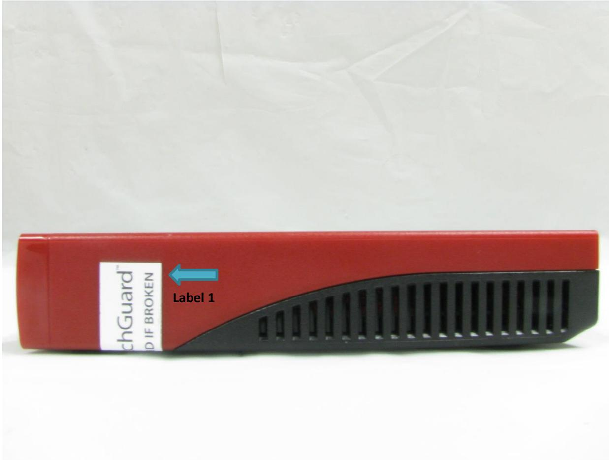
Figure 16: T10-W Tamper Evident Label 1 Placement
