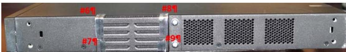
Figure 7-10: Tamper Seal Locations - Right Side Ventilation Cover
