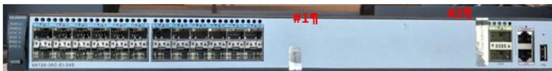
Figure 7-8: Tamper Seal Locations - Front
