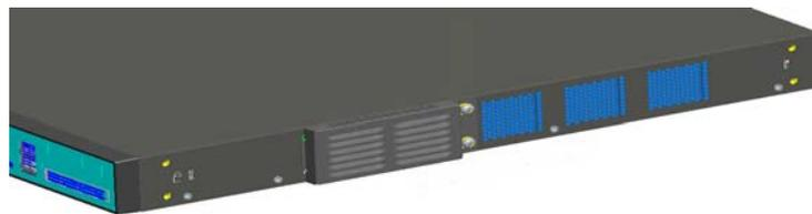
**Figure 7-6: Gently push the baffle to fit the tabs in the air vents. Use two M4\*8 screws to affix the baffle.**
