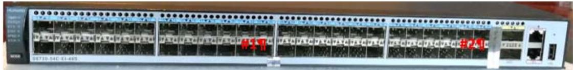
Figure 7-12: Tamper Seal Locations - Front
