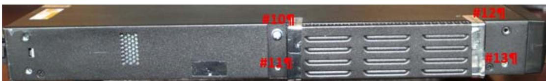
Figure 7-11: Tamper Seal Locations - Left Side Ventilation Cover
