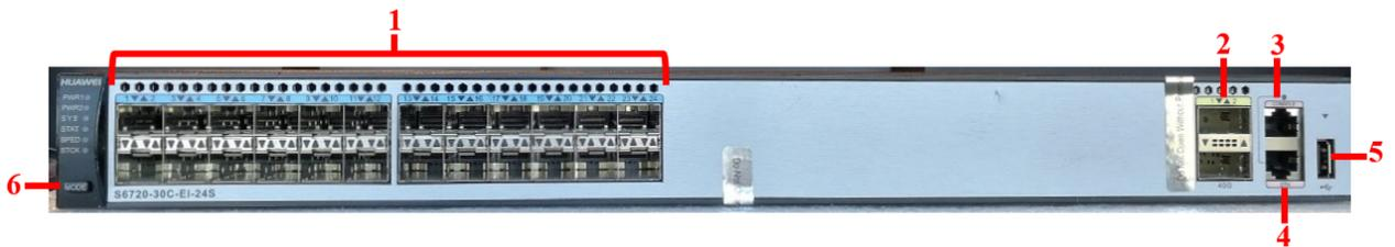
Figure 3-1: S6720-30C-EI-24S-AC Ports – Front Panel
