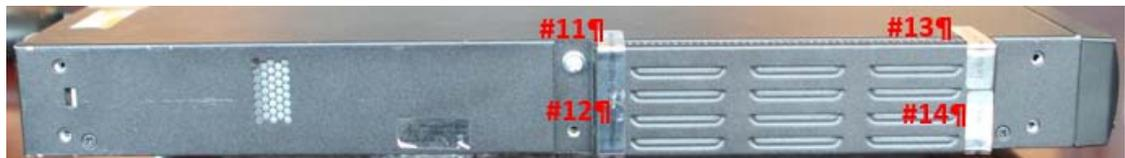
Figure 7-15: Tamper Seal Locations - Left Side Ventilation Cover
