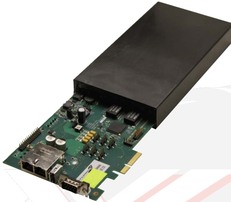
Figure 2 – GSP3000 with its Tamper Potting Intact
