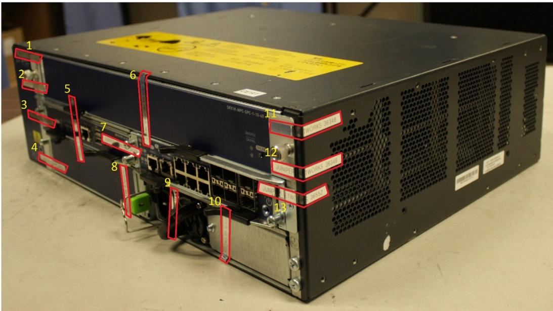
**Figure 10: SRX1400 Tamper-Evident Seal Placement on Front & Right Side-13 Tamper Seals**
