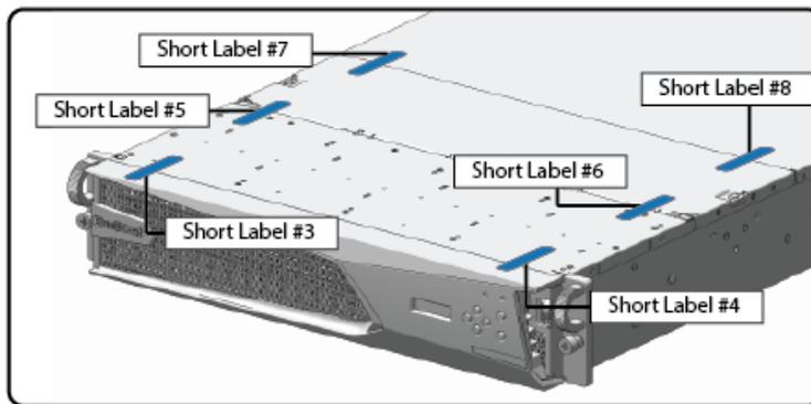
**Note:** The chassis-center cover labels are destroyed each time the center cover is opened. Be sure to re-secure the appliance after servicing!
