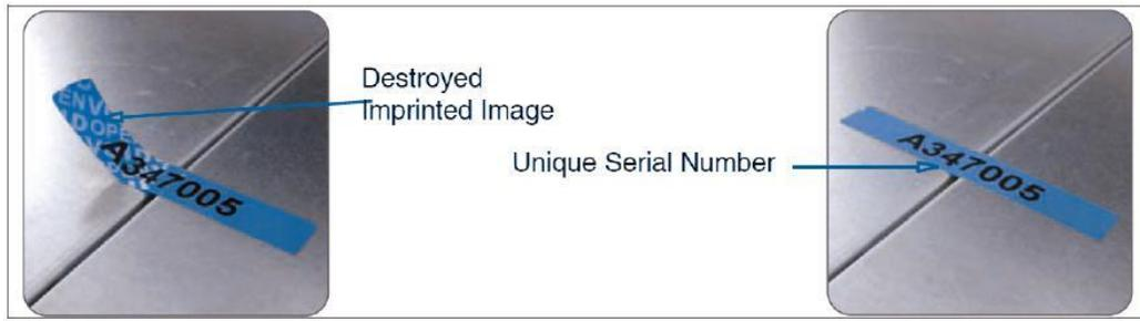
**Figure 8 Labels Showing Tamper Evidence**
