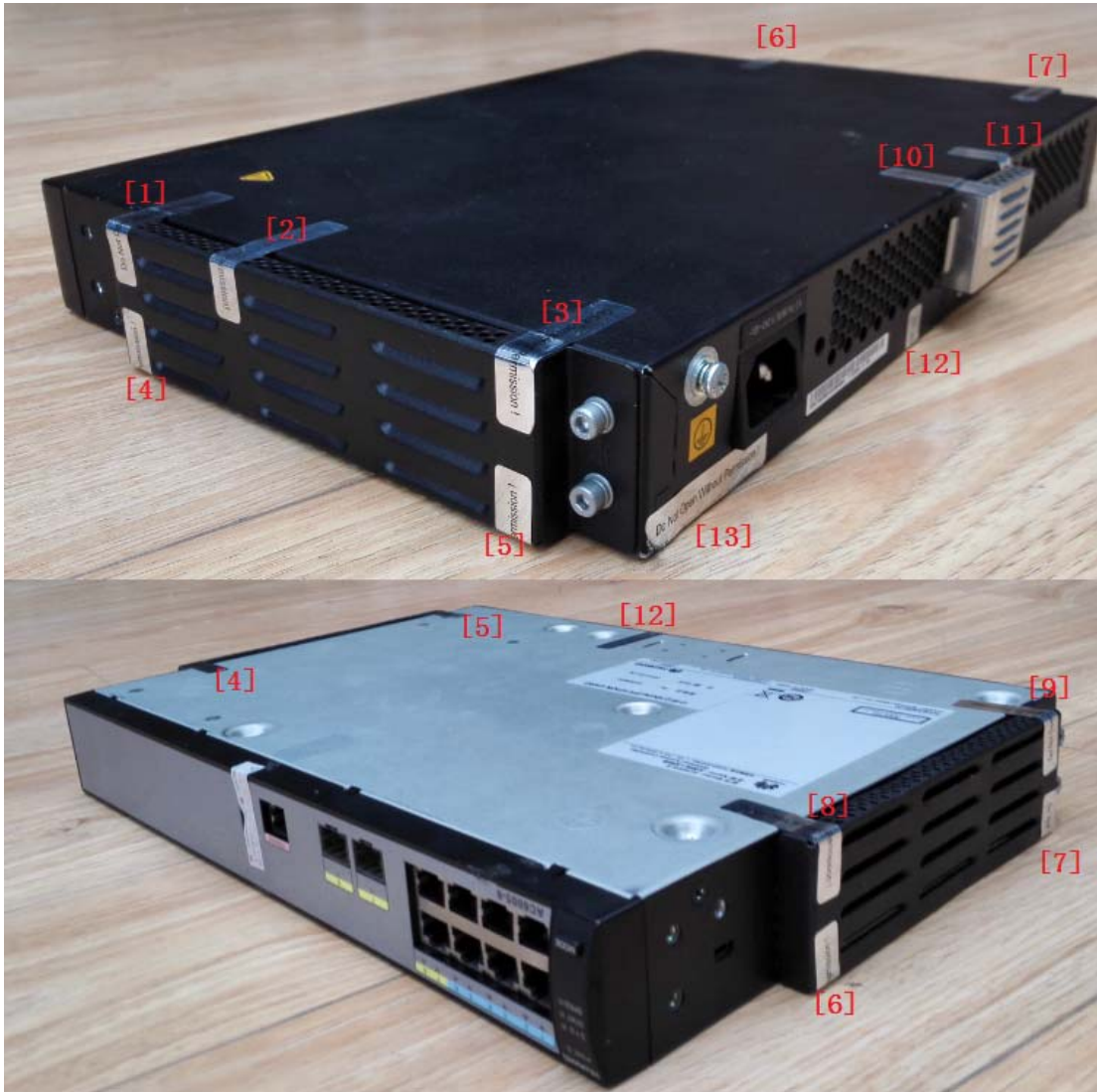
Figure 3 - AC6005 Tamper-evident Seal Placement
