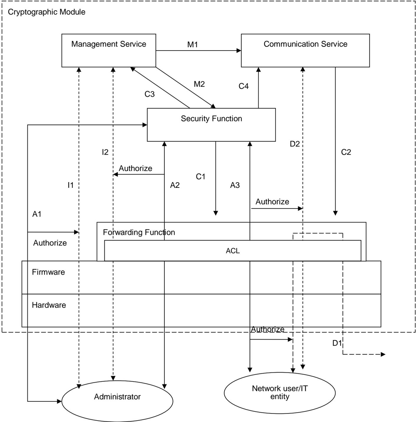
**Figure 1 Security Architecture Block Diagram**
