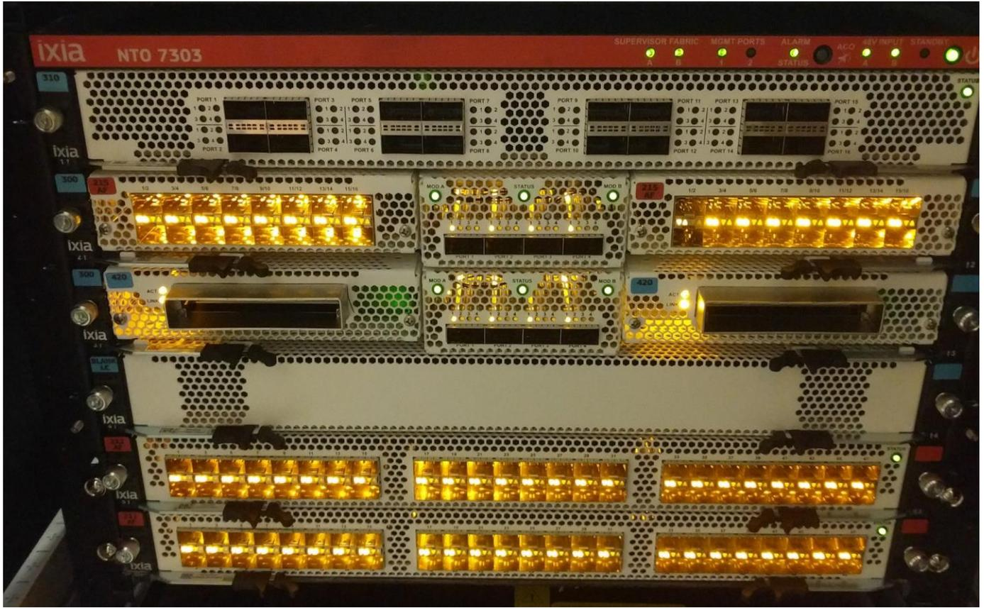
Figure 1 – NTO 7303 Chassis P/N 991-0082-01 (Front view; fully populated)
