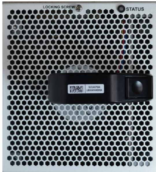
Figure 13 – NTO 7300 Series Fan Module Unit P/N 991-2013-01
