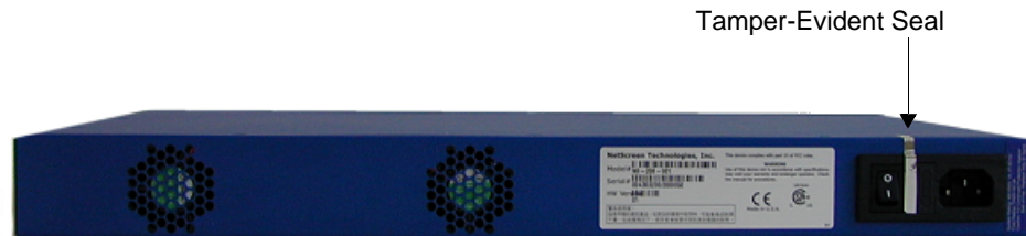
Figure 3 Tamper-Evident Seal on AC Interface
