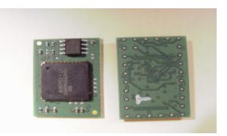
The SEM can be incorporated into any radio device, which requires FIPS 140-2 Level 1 cryptographic security functionality.
