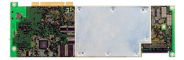
Figure 2: Vortex Secure Card back. The crypto boundary is defined by the metallic shield.
