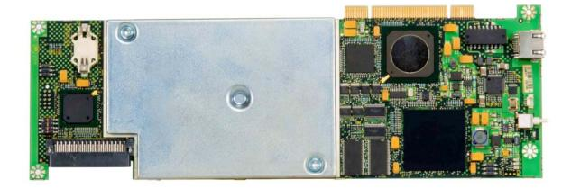
Figure 1: Vortex Secure Card front. The crypto boundary is defined by the metallic shield.
