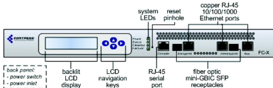
Figure 3: Front View of the FC-X
