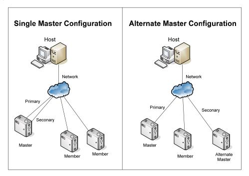
Figure 3 – Single and Alternate Master Configurations
