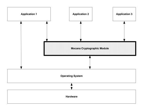
Figure 1 – Cryptographic Module Interface Diagram
