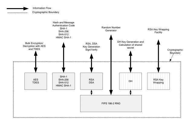
Figure 2 – Logical Cryptographic Boundary
