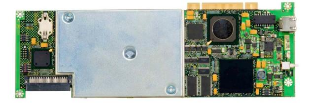
Figure 1: MCC7500 Secure Card front. The crypto boundary is defined by the metallic shield.
