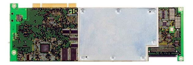
Figure 2: MCC7500 Secure Card back. The crypto boundary is defined by the metallic shield.
