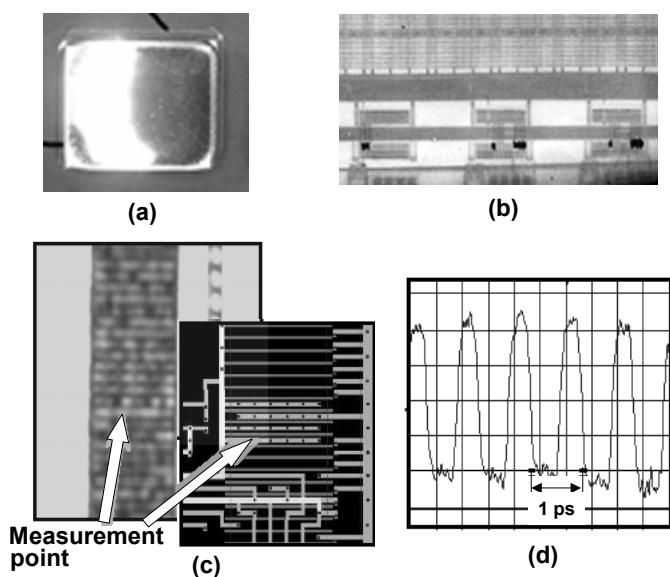
**Fig. 8 Measurement of waveform from backside by LVP.**
