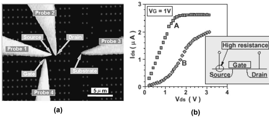
**Fig. 11 Measurement of DC characteristics of a MOSFET in a sRAM cell by using a nano-prober: (a) photograph of probes contacting to via plugs, (b) Measured I-V characteristics (A: normal, B: abnormal).**
