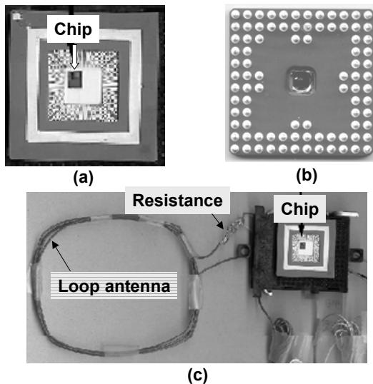
**Fig. 15 Packaged removed chip and build-up spurious IC card with loop antenna connected to package. The spurious IC card operates as well as real non-contact IC card.**
