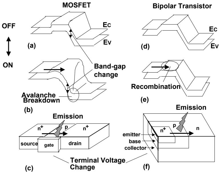
Fig.1 Physical phenomena generated in operating MOSFETs and bipolar transistors.
