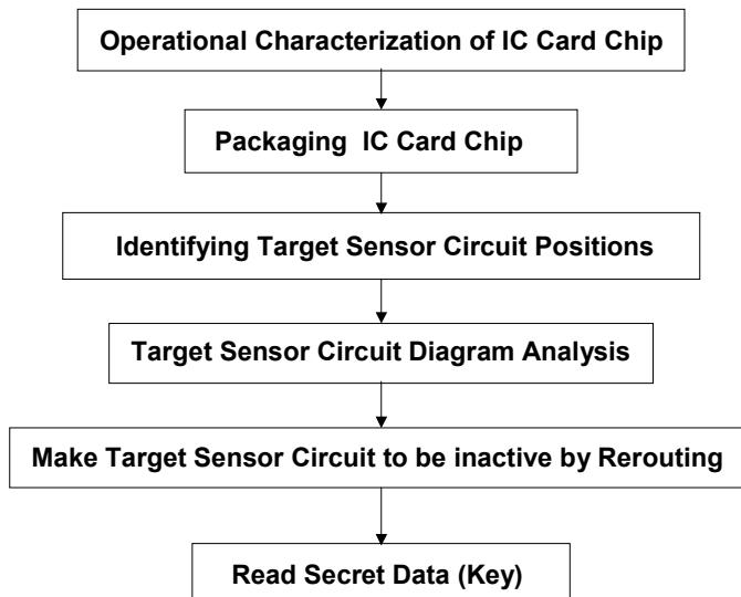
Fig. 13 A Flow of Physical Attack
