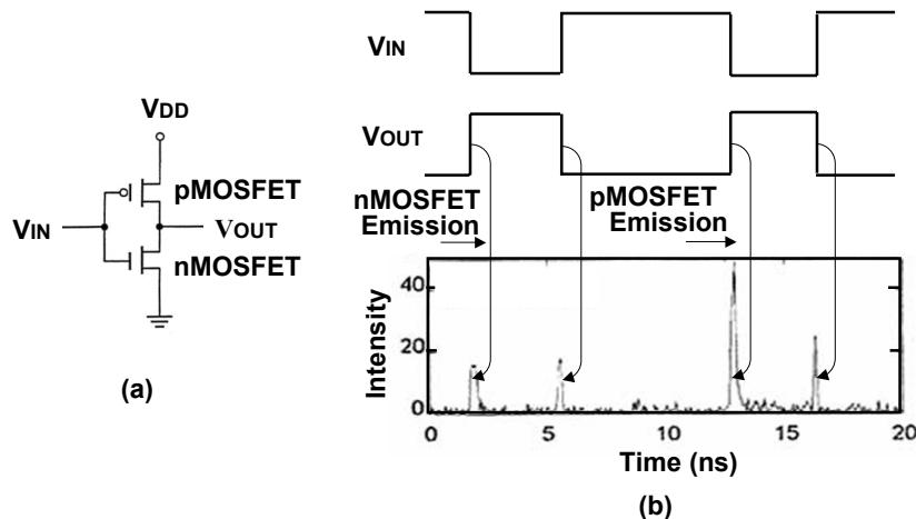
**Fig. 9** Measurement of photon emission from backside: (a) circuit diagram of CMOS inverter and (b) detected time resolved photon emission from CMOS inverter by TRE.
