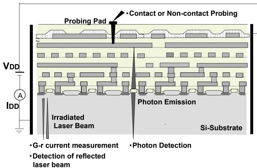
Fig.3 Typical methods to detect physical phenomena in LSIs.
