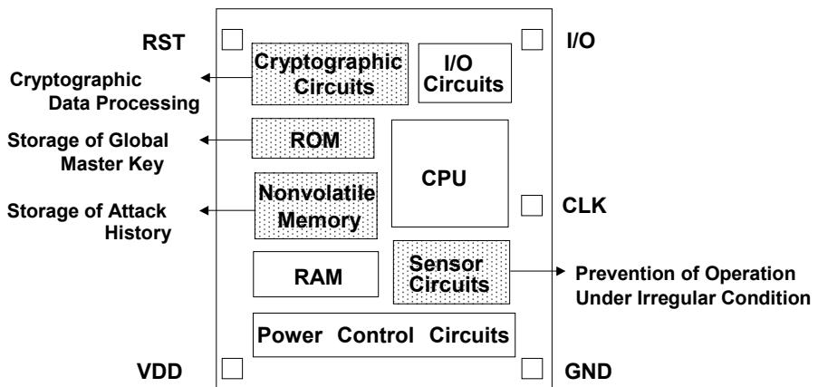
**Fig. 12 Basic block diagram of IC card Chip with general target blocks for physical attacks shown as dotted blocks.**
