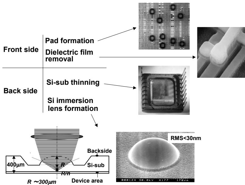
Fig. 5 Sample preparation techniques for operating waveform measurements.
