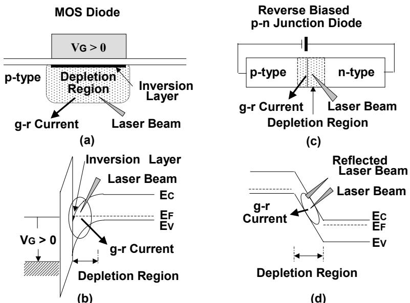
Fig.2 Generation-recombination current flow in depletion region by laser beam irradiation. Polarization of reflected laser beam is varied with electric field strength in operating device due to Frantz-Keldish effect.
