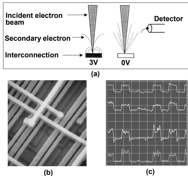
**Fig. 7 Measurement of waveforms from front-side by EBT.**
