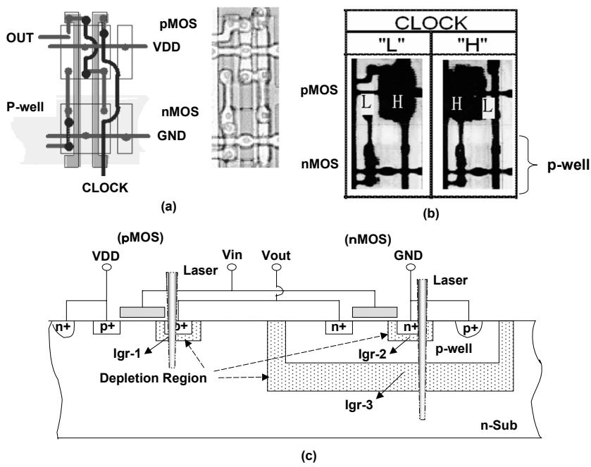
Fig. 6 Observation of “H” or “L” state of node by OBIC.
