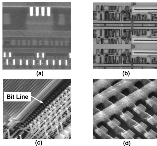
Fig. 4 Sample preparation techniques for structural analysis of LSIs: (a) cross-section formation by FIB, (b) successive metal layer lapping, (c) & (d) interlayer dielectric film removal by wet etching.
