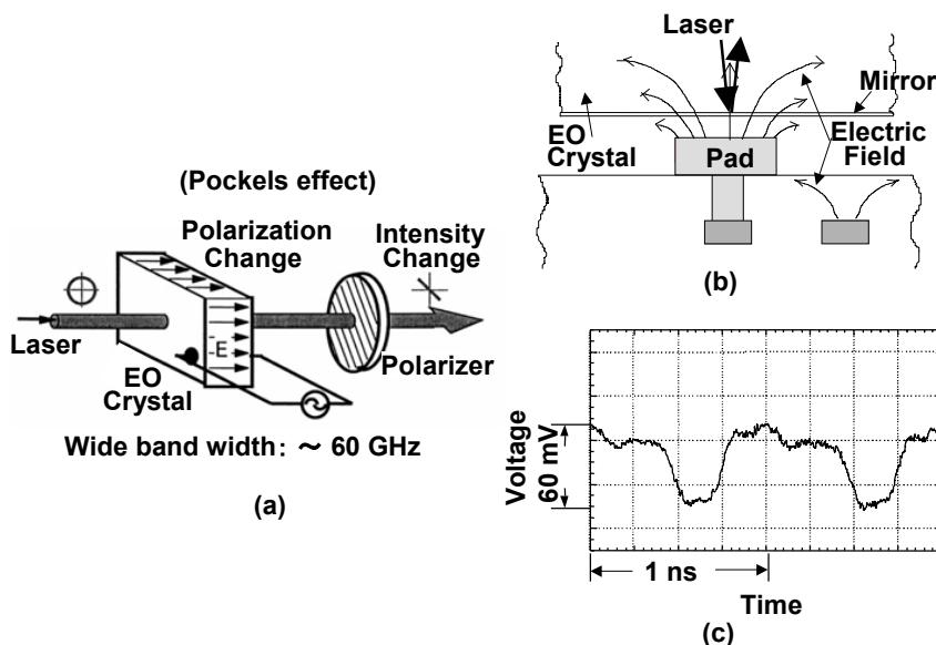
**Fig. 10** Principle of EO-sampling and result of high speed and low Voltage signal measurement.
