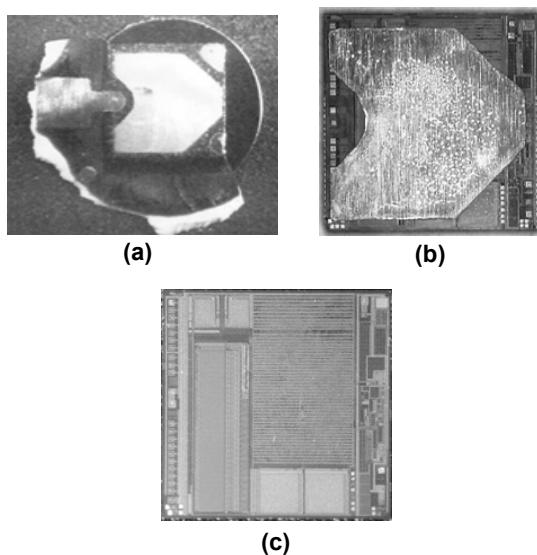
Fig. 14 Flow of chip removal from IC card ((a) to (c)).
