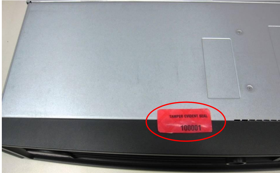
Figure 12 – WG5000 Front Bezel Seal Placement (Top)
