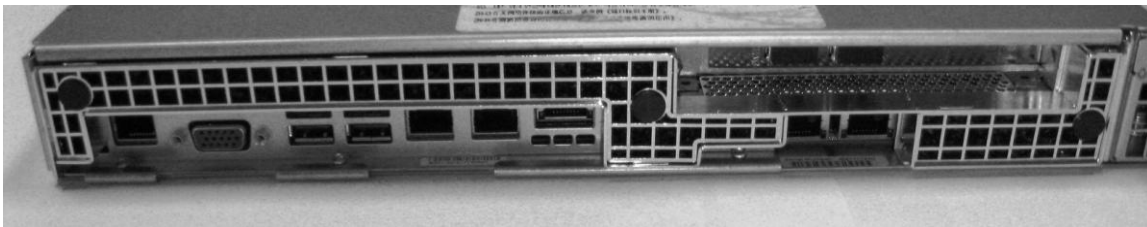
Figure 9 – Opacity Baffle Installed on WG5000
