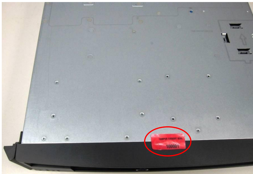
Figure 17 – WG5500 Front Bezel Seal Placement (Bottom)
