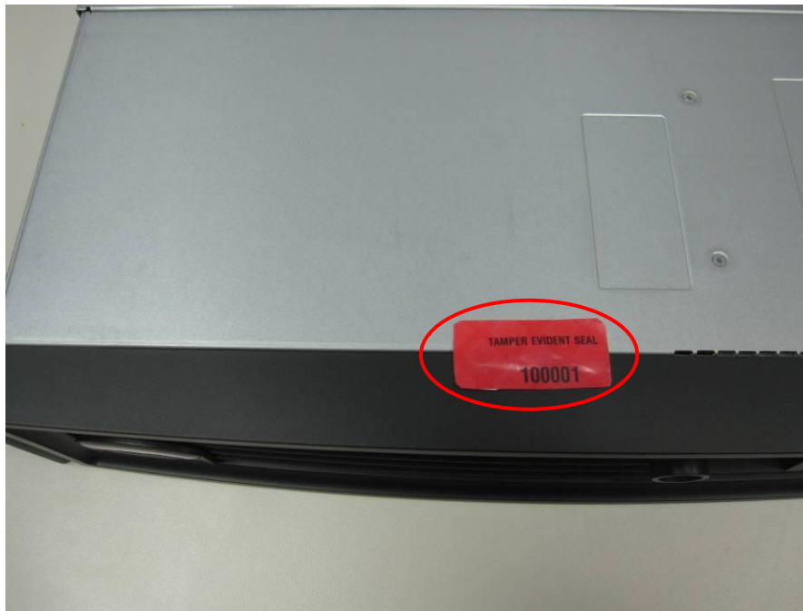
Figure 15 – WG5500 Front Bezel Seal Placement (Top)
