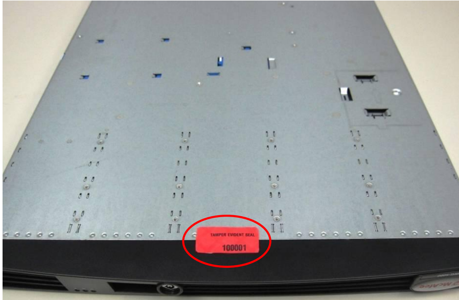
Figure 14 – WG5000 Front Bezel Seal Placement (Bottom)
