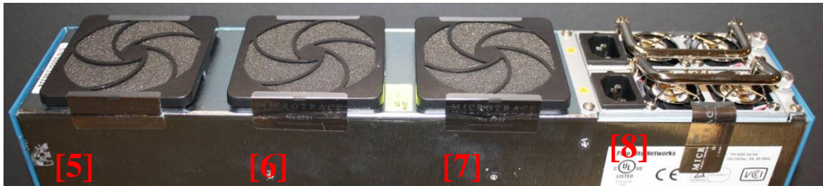
Figure 27 - PA-4000 Series Rear Side Tamper Seal Placement – From Underside (4)
