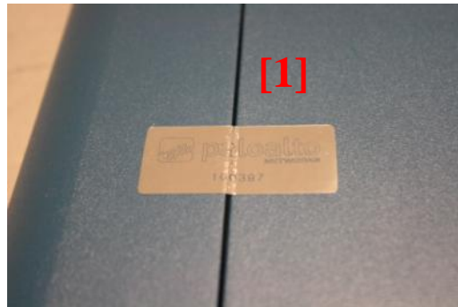
Figure 18 - PA-500 Front Tamper Seal Placement (1)
