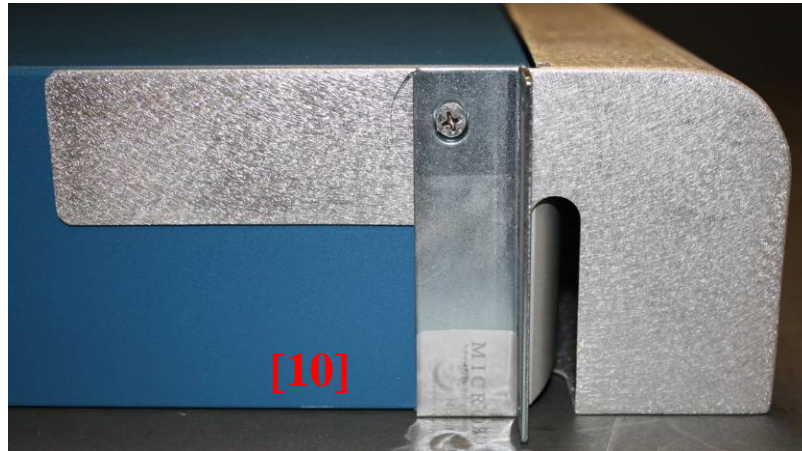
Figure 29 - PA-4000 Series Left Side Tamper Seal Placement (1)
