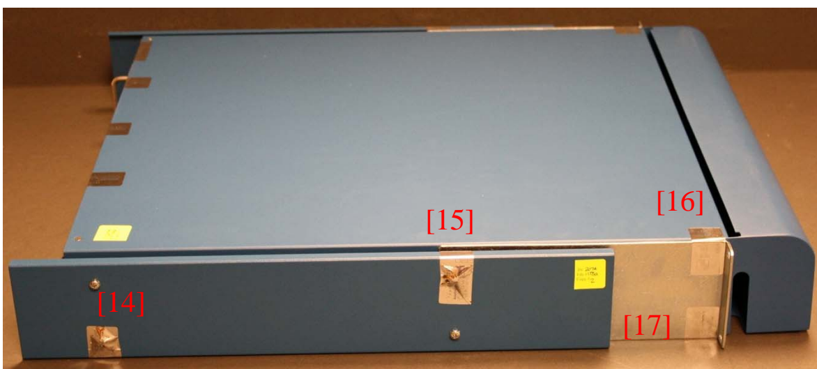
Figure 32 - PA-5000 Series Left Side Tamper Seal Placement (4)
