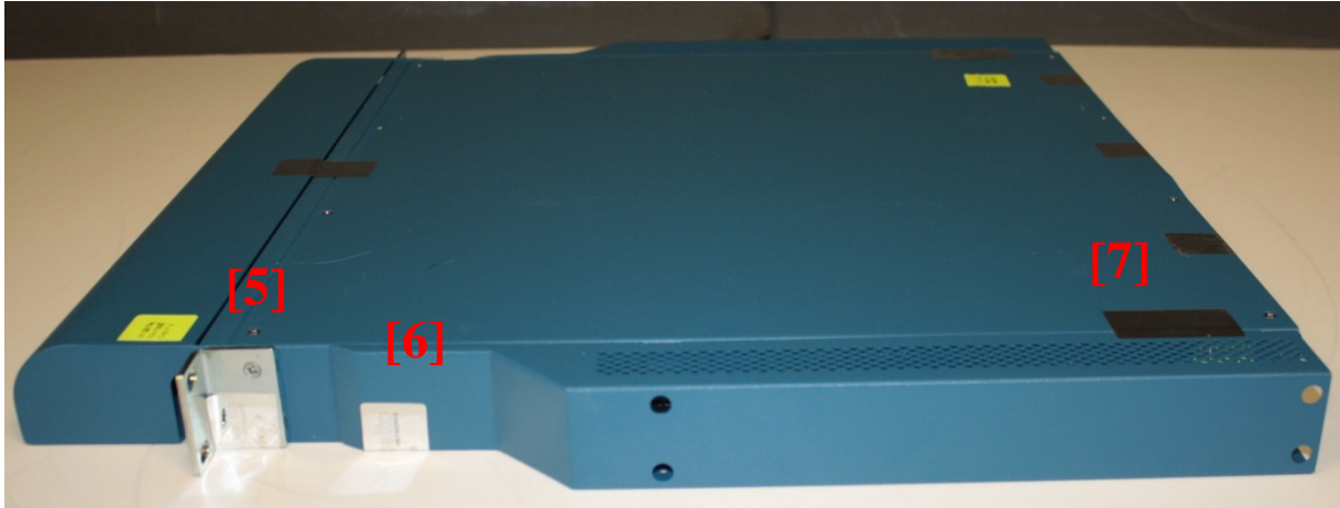
Figure 24 - PA-2000 Series Right Side Tamper Seal Placement (3)
