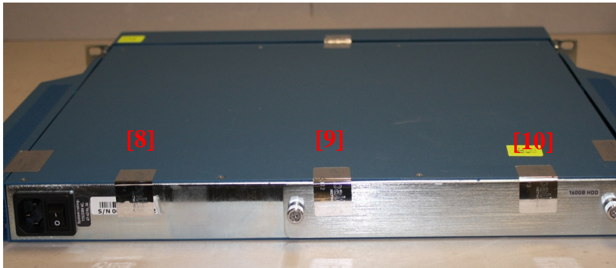
Figure 25 - PA-2000 Series Rear Tamper Seal Placement (3)
