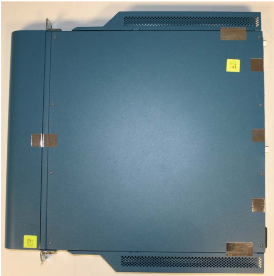
Figure 7 - PA-2020 / PA-2050 Front Opacity Shield
