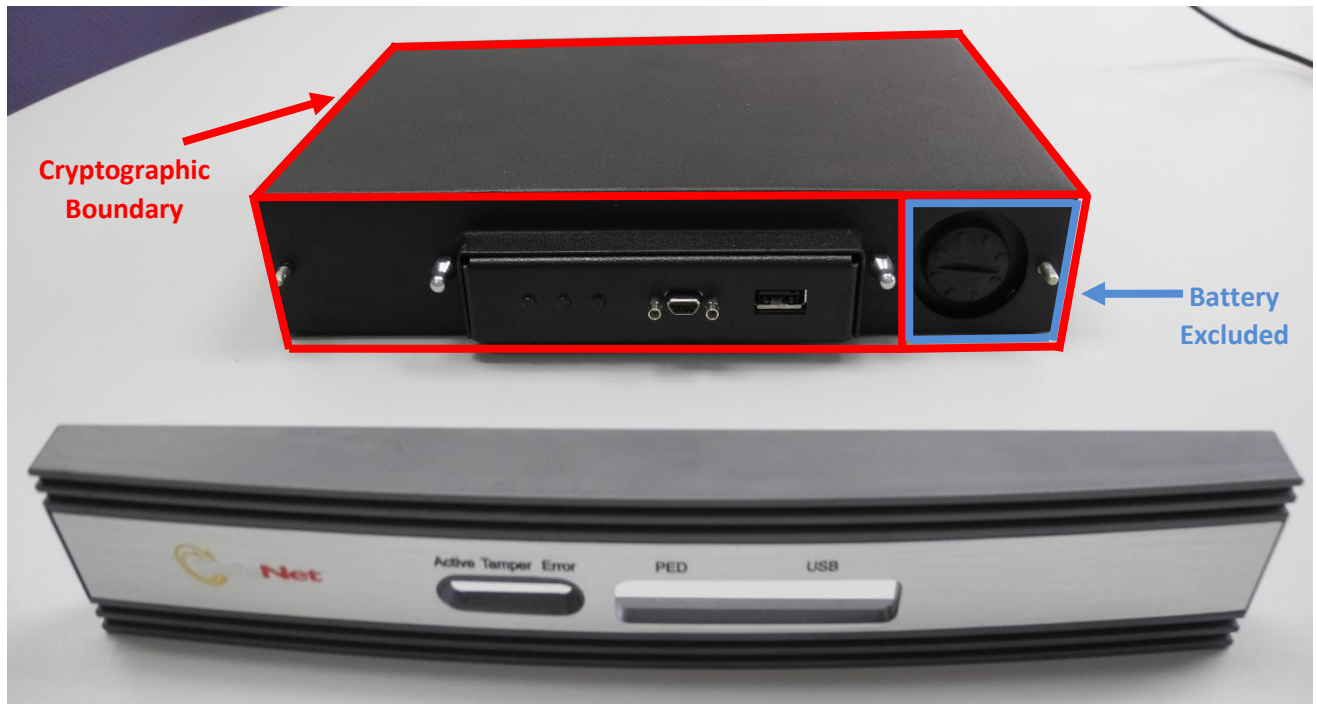
Figure 2-2. Luna G5 Cryptographic Boundary (with front bezel removed)
