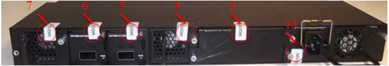
Figure 55. Rear side of the Brocade® ICX 7450. In addition to labels 3, 4, 5, 6, and 7 that were described in Figure 57, (Qty. 1) TEL is utilized to secure the power supply to the bottom of the module (label 13).
