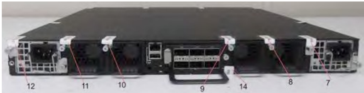
Figure 51 Rear top view of Brocade ICX 7750 device with security seals
