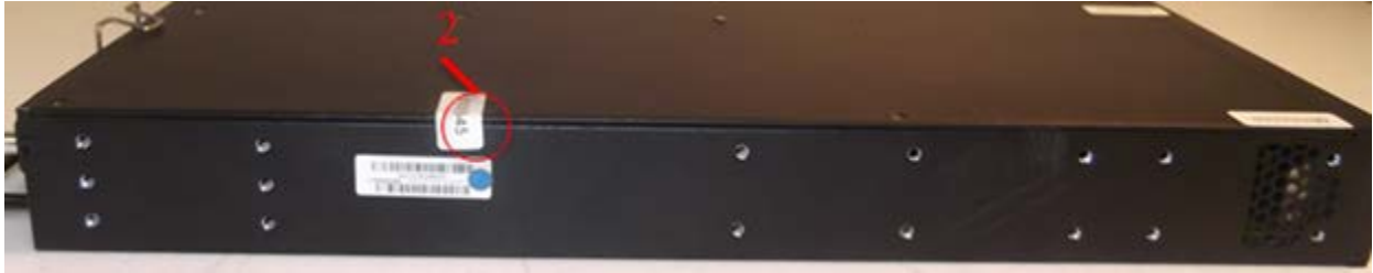
Figure 56. Left side of the Brocade® ICX 7450. (QTY.1) TEL is placed on the left side (label 2), and secures the top covers to the left side of the module.
