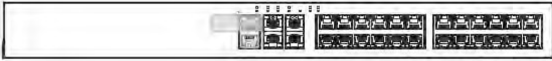
Figure 43 Security Seal over the console port on the Brocade ICX 6450-48 and ICX 6450-48P devices
