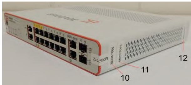
Figure 46 Front right side view of a Brocade ICX 6450-CP12-PD device with security seals
