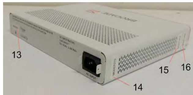
Figure 48 Back left side view of a Brocade ICX 6450-CP12-PD device with security seals
