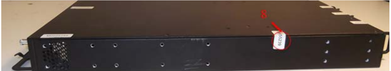
Figure 57. Right side of the module Brocade® ICX 7450. (QTY. 1) TEL is placed on the right side (label 8), and secures the top cover to the right side of the module.
