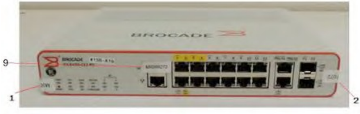
Figure 46 Front right side view of a Brocade ICX 6450-CP12-PD device with security seals
