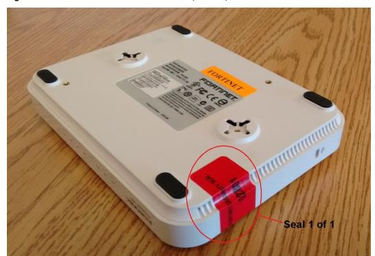
Figure 7: FortiGate-30D external enclosure seal, bottom, left side
