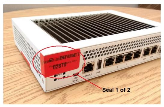
Figure 11: FortiGateRugged-60D front panel seal
