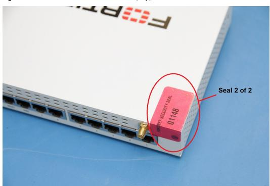
Figure 9: FortiWifi-60D external enclosure seal, top, rear
