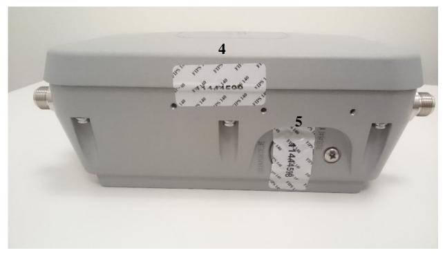
Cisco Aironet 1562e/d/ps tamper label placement (Front, Back, Left, Right)
