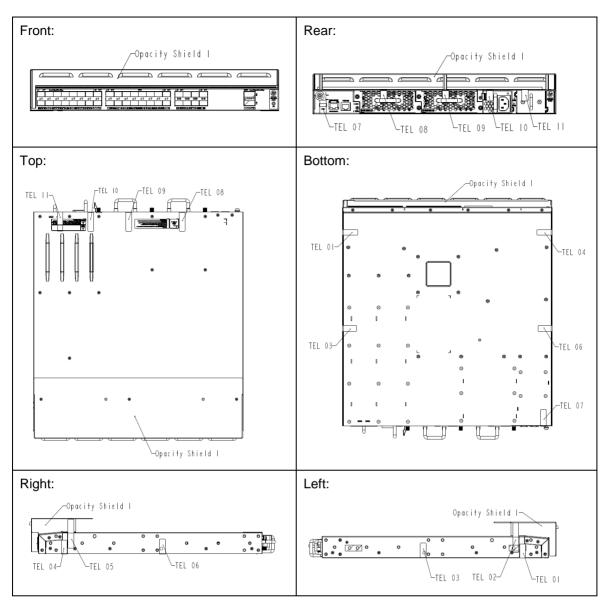
Figure 6 HPE FlexFabric 5700-40XG-2QSFP+ Switch (JG896A) / HPE FlexFabric 5700-40XG-2QSFP+ TAA1-Compliant Switch (JG897A) Tamper Evidence Labels and Opacity Shields
