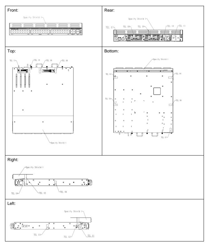
Figure 13 HPE FlexFabric 5900AF-48G-4XG-2QSFP+ Switch (JG510A) / HPE FlexFabric 5900AF-48G-4XG-2QSFP+ TAA1-Compliant Switch (JH038A) Tamper Evidence Labels and Opacity Shields
