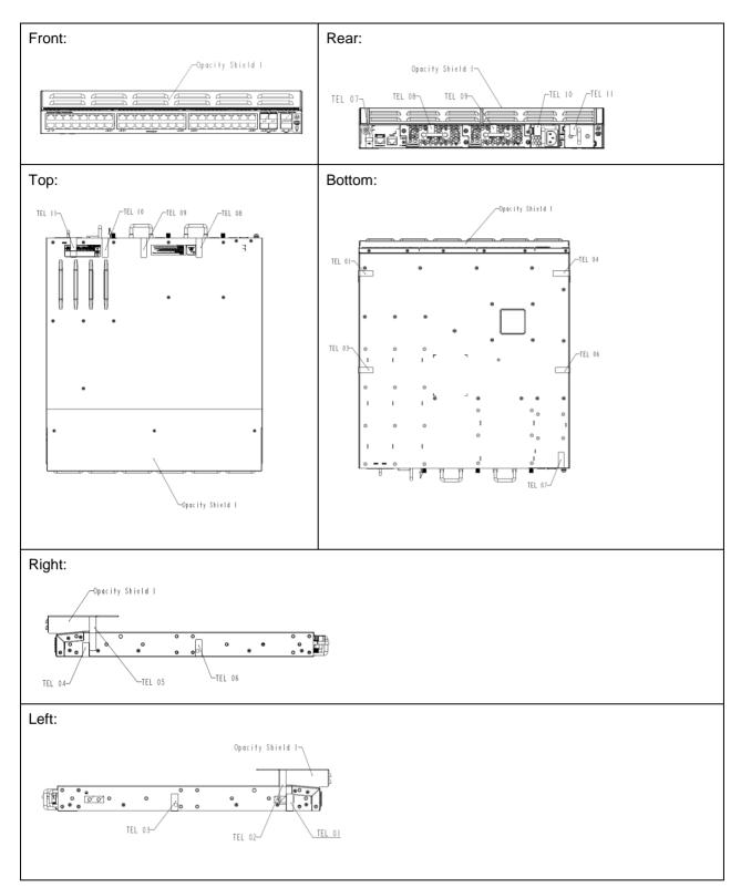
Figure 7 HPE FlexFabric 5700-48G-4XG-2QSFP+ Switch (JG894A) / HPE FlexFabric 5700-48G-4XG-2QSFP+ TAA1-Compliant Switch (JG895A) Tamper Evidence Labels and Opacity Shields
