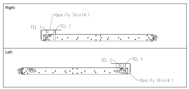
Figure 17 HPE FlexFabric 5920AF-24XG Switch (JG296A) / HPE FlexFabric 5920AF-24XG TAA-compliant Switch (JG555A) Tamper Evidence Labels and Opacity Shields
