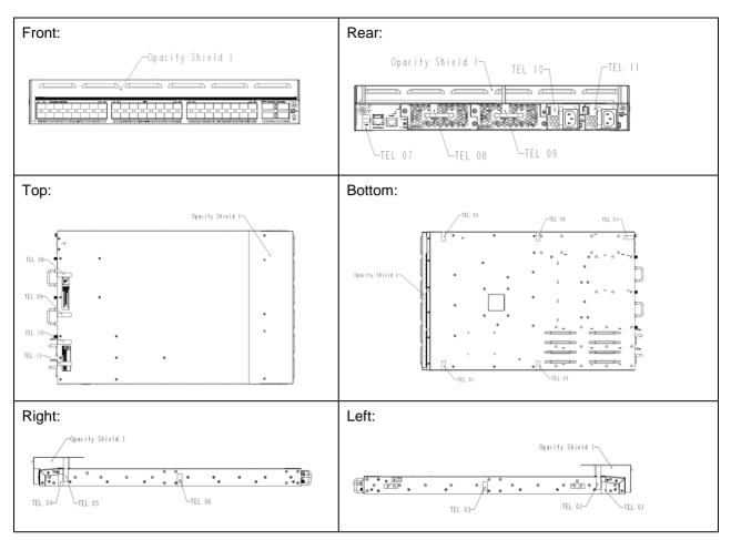
Figure 12 HPE FlexFabric 5900AF-48XG-4QSFP+ Switch (JG772A) / HPE FlexFabric 5900AF-48XG-4QSFP+ TAA1-Compliant Switch (JG554A) Tamper Evidence Labels and Opacity Shields
