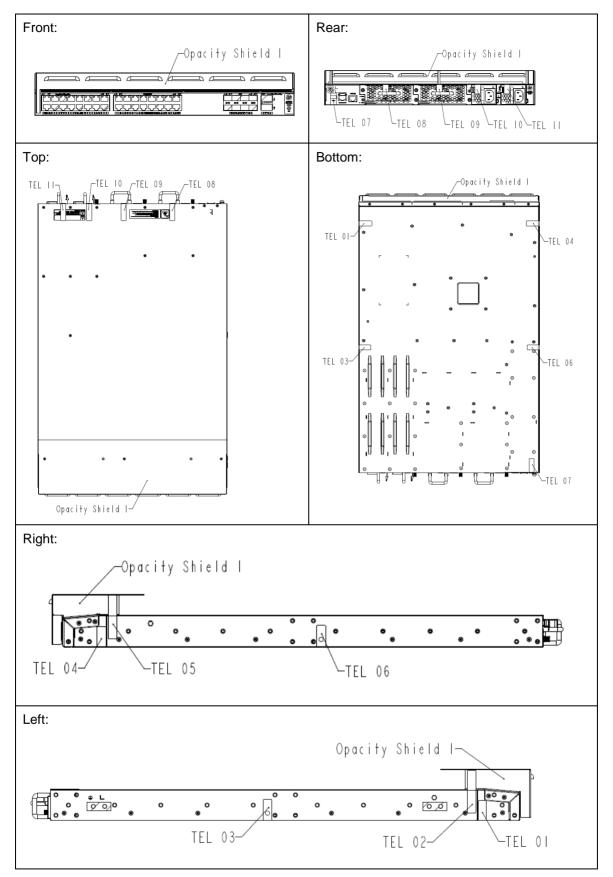
Figure 5 HPE FlexFabric 5700-32XGT-8XG-2QSFP+ Switch (JG898A) / HPE FlexFabric 5700-32XGT-8XG-2QSFP+ TAA -Compliant Switch (JG899A) Tamper Evidence Labels and Opacity Shields
