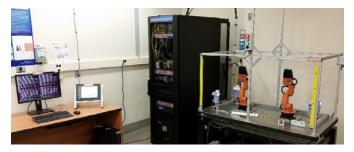
Figure 8: Collaborative robotics portion of the ICS cybersecurity testbed
