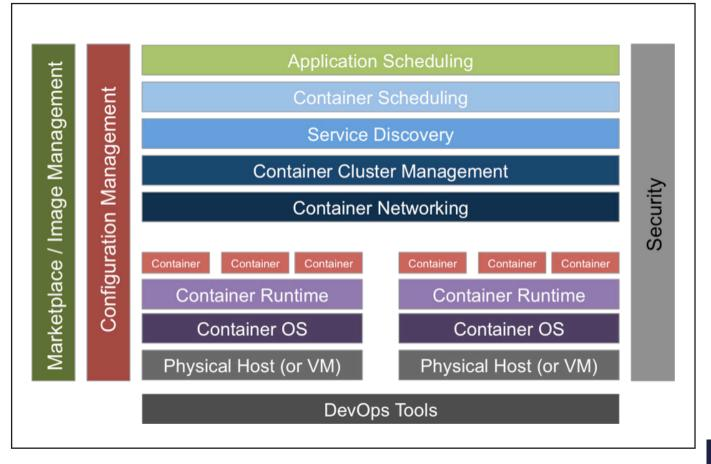
Figure 32: Container Technology Stack
